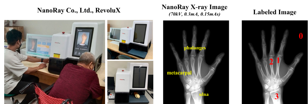
Figure 8. RevoluX X-ray machine and its corresponding annotated images, which include the background, 2MC, 3MC, and radius, are labeled as 0, 1, 2, and 3, respectively.
