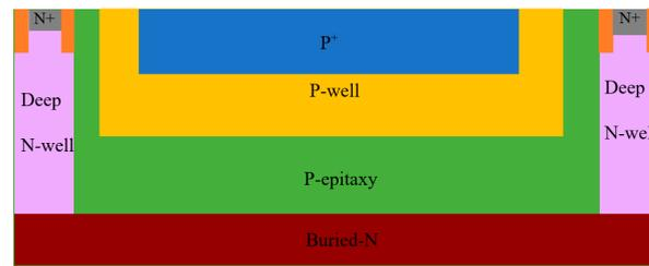
**Figure 2.** Cross-section of the P-I-N-structure SPAD.
