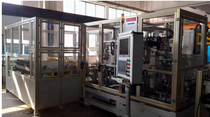
**Figure 6.** Connecting rod online measurement machine.
