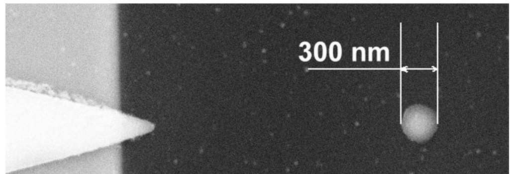
Figure 8. SEM image of a 50 nm thick SiN membrane with a 300 nm permalloy nanodisk.
