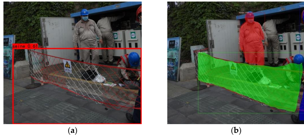
Figure 1. The results of irregular deformable object detection using different detectors. (a) The horizontal rectangle; (b) The polygonal bounding box.
