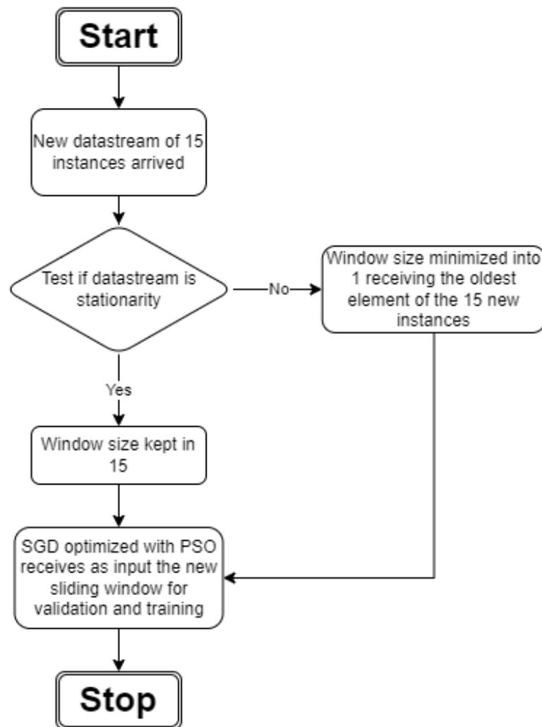
**Figure 8.** The proposed method flowchart.
