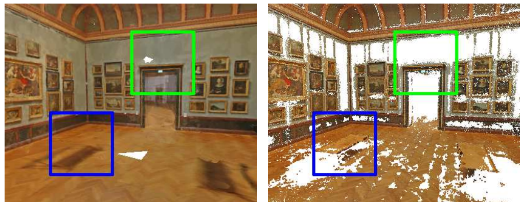
Figure 3. CPMVS (left) can successfully reconstruct the textureless regions (the green square), while PMVS (right) can capture small details such as the benches (the blue square).
