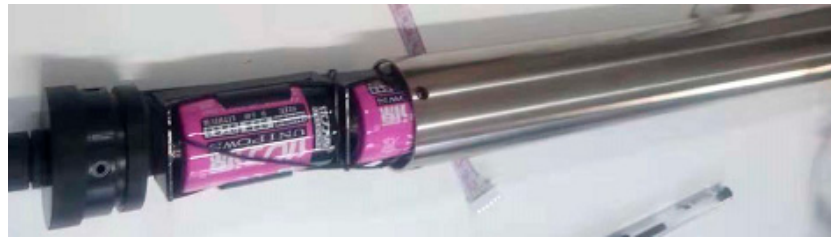
Figure 11. The 48 mm steel-pipe installation of an NB-IoT-based D/RTU, used by EMULSION.
