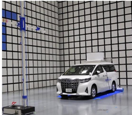
**Figure 1.** E-field measuring equipment in a radome mounted on a car in an anechoic chamber.
