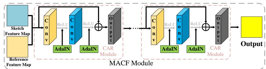
**Figure 3.** The proposed multi-level adaptive-instance-normalized color fusion (MACF) consists of four identical CAR modules. Given a set of sketch and reference images, different results are output by level-by-level CAR. It is a multi-level operation that enables the natural fusion of color features with sketch features.
