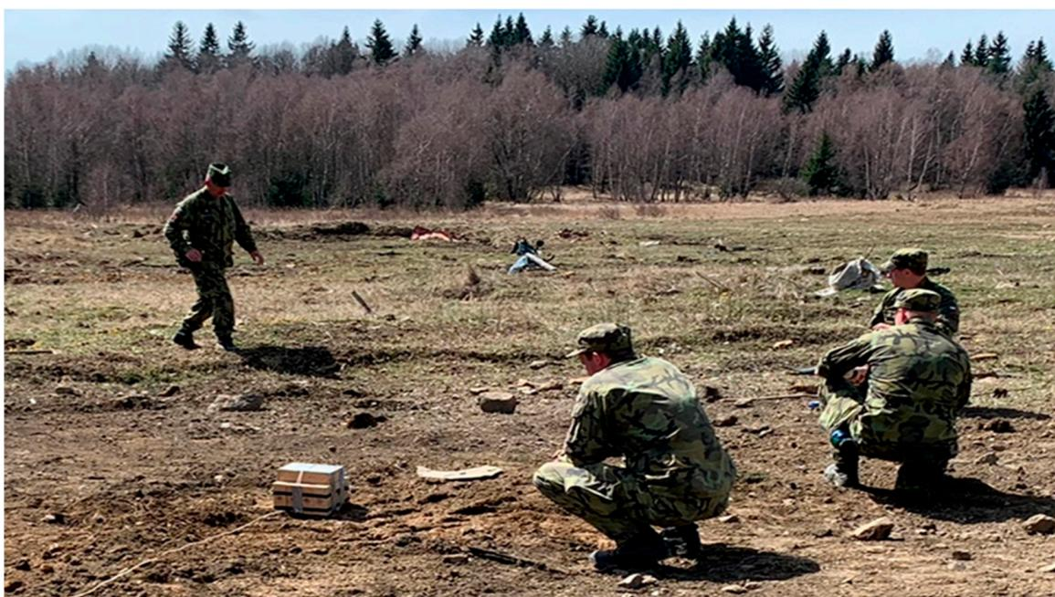
**Figure 12.** Installation of a TNT charge and an optical fiber sensor for measuring 5 kg of TNT (Boletice Military Training Area, Pražačka Artillery Pit).
