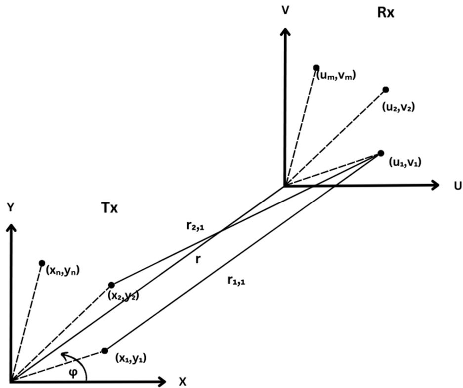
Figure 3. Schematic diagram of the MIMO antenna on XY and UV coordinate planes.
