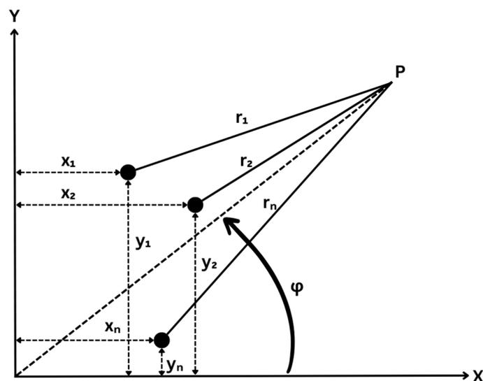
Figure 4. Schematic diagram of dipole placement in XY coordinate plane.
