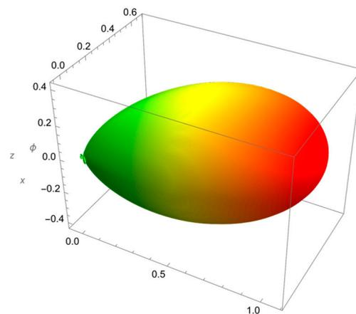
**Figure 7.** Three-dimensional view of the single beam formed at  $30^\circ$  when the transmitter antenna elements are half-wave dipoles.
