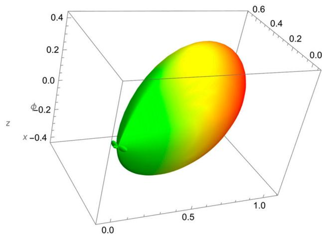
**Figure 10.** The same beam is shown at an angle for a better view of the side lobes. The side lobes have negligible energy.
