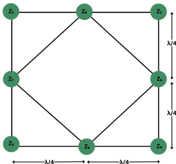
**Figure 5.** Proposed eight-element dipole antenna.
