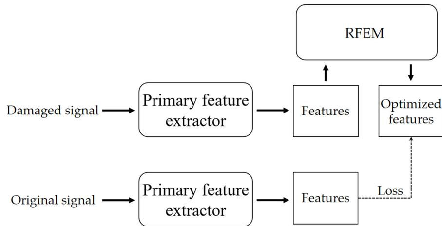
Figure 6. Schematic diagram of anti-noise task.
