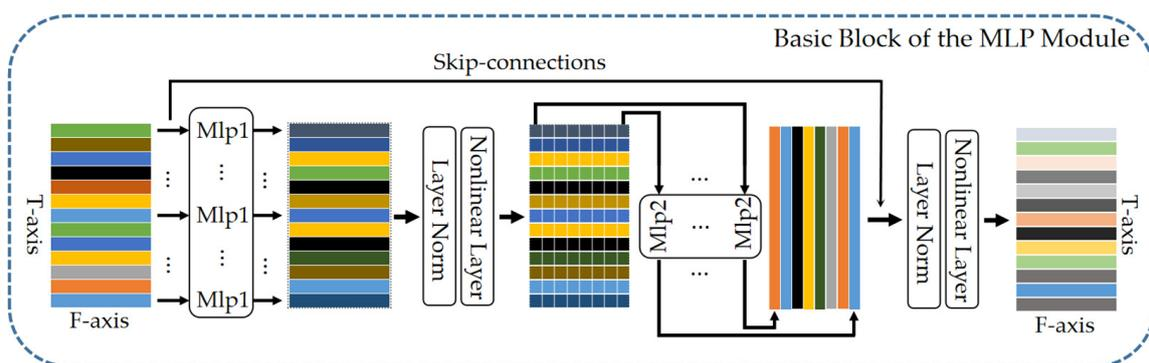
**Figure 3.** Schematic diagram of basic block of the MLP module.
