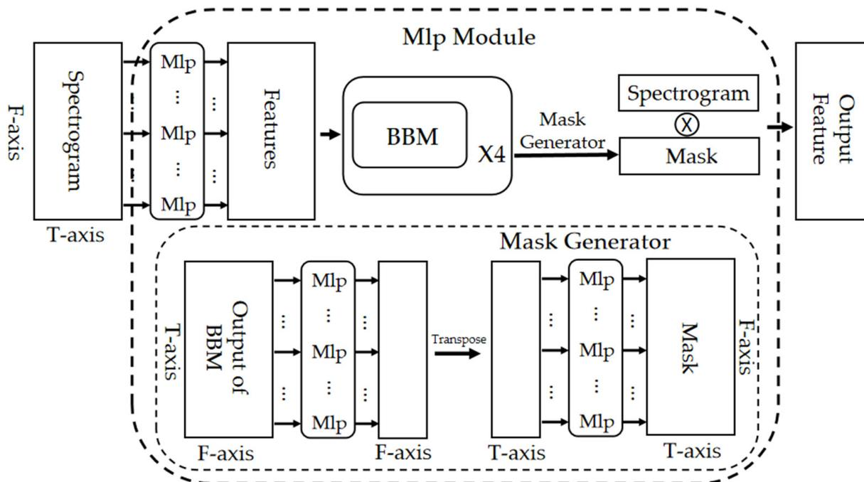
Figure 4. Schematic diagram of the MLP module.
