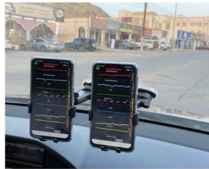
Figure 4. Smartphones mounted in moving vehicles during drive test [40].
