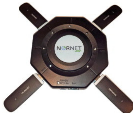
Figure 8. NNE node with 4 modems connected [52].
