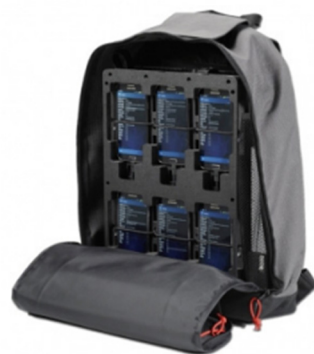
Figure 5. Bag pack with six mounted smartphones.
