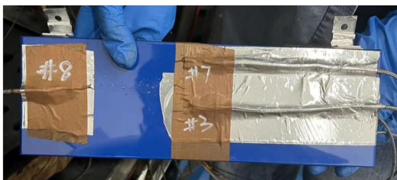
**Figure 3.** Thermocouple paste method diagram.
