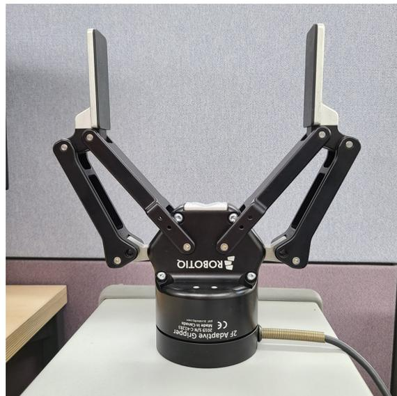
**Figure 3.** The gripper used in the proposed system is Robotiq's 2F-140 gripper.
