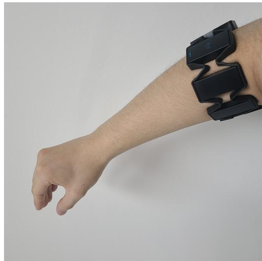
**Figure 6.** Band-shaped sensor worn on the user’s right forearm. Channel 4 should be aligned horizontally with the back of the user’s hand.
