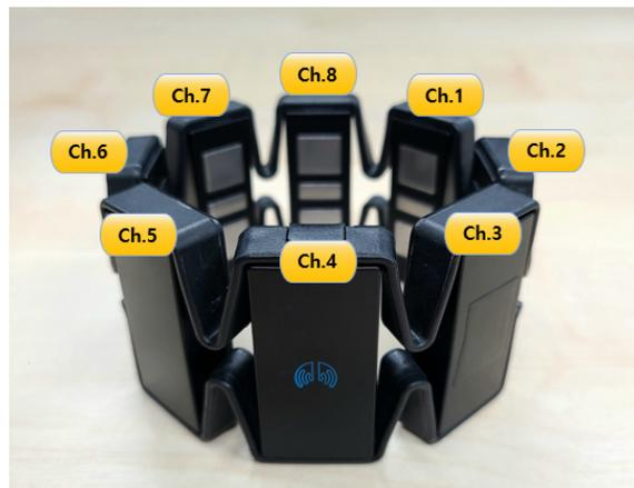
**Figure 4.** Myo gesture control armband EMG sensor used in this study. The wearable device has eight surface EMG channels.
