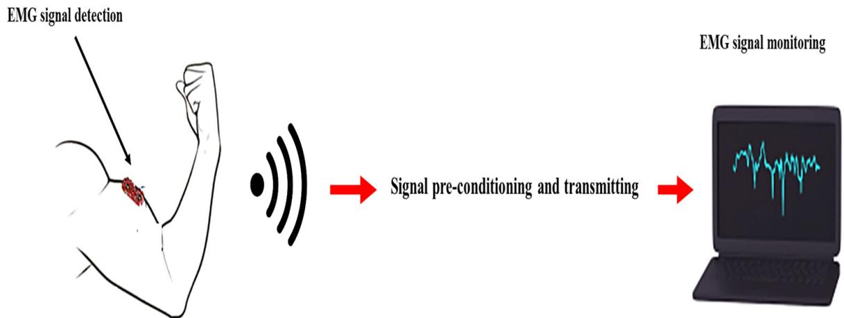
Figure 4. EMG monitoring system structure.
