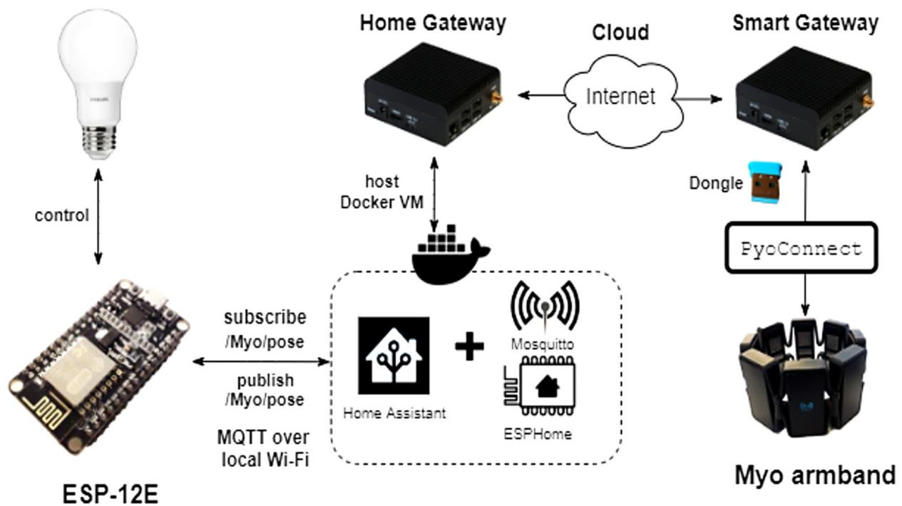
Figure 6. Architecture of the EMG-based control system proposed in [113] (Reproduced with permission from [113], IEEE, 2021).
