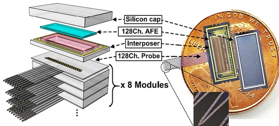
**Figure 7.** Proposed IC in [114]: Conceptual diagram of a 1024-channel parallel-recording platform assembled with the proposed 128-channel AFEs, interposers, silicon caps, and 128-channel multi-shank probes, and a photograph of the fabricated module on the top of a U.S. penny (Reproduced with permission from [114], IEEE, 2018).
