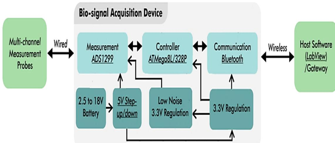
**Figure 8.** Device architecture proposed in [118] (Reproduced with permission from [118], IEEE, 2017).
