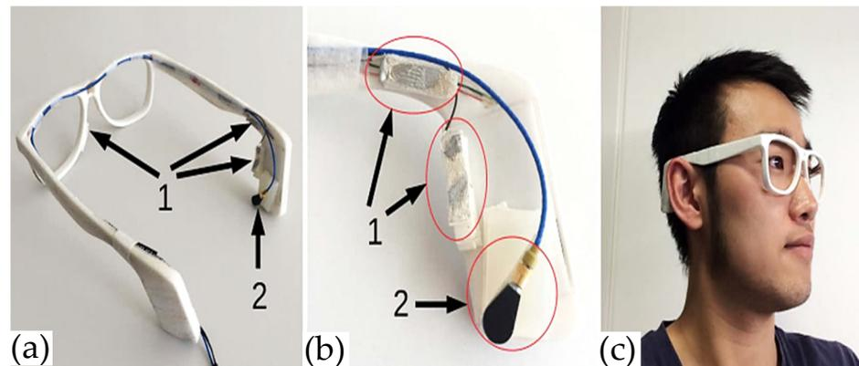
**Figure 9.** Prototype of the 3D-printed smart glasses, presented in [120] (a) with integrated bone vibration sensor and EMG electrodes applied on the right temple (b). Smart eyeglasses worn by a user (c) (Web-source: <https://dl.acm.org/doi/10.1145/2971763.2971799>, every aspect related to the human sub-jects' involvement has been taken into consideration by the authors in [120]) (Image courtesy by the authors, R. Zhang and O. Amft [120]).
