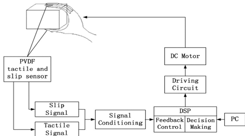
**Figure 2.** Schematic of the prosthetic hand control system presented in [93] (Reproduced with permission from [93], IEEE, 2012).
