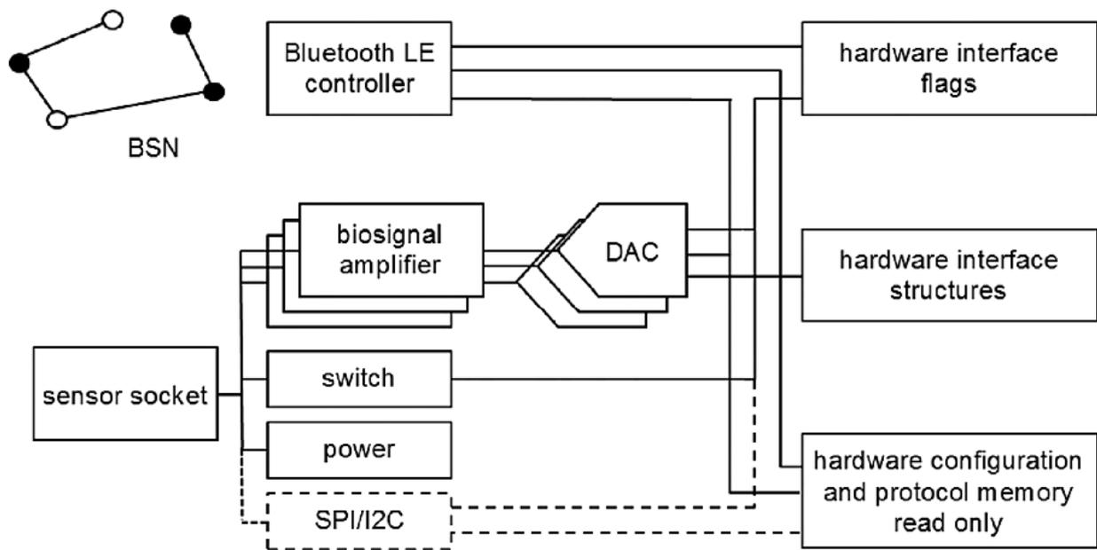
**Figure 12.** Flow diagram of the data acquisition layer proposed in [129] (Reproduced with permission from [129], Elsevier, 2016).
