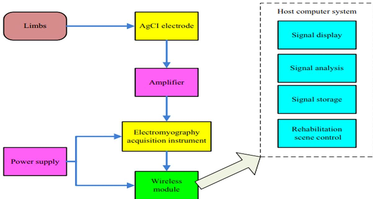
**Figure 3.** Flowchart of electromyography acquisition system [101] (Reproduced with permission from [101], Springer Nature, 2019).
