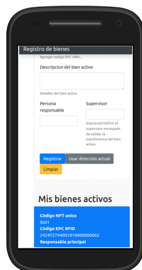
Figure 12. Chainway C72 RFID UHF GEN II portable reader, mobile DAPP showing the form to register new assets and the list of assets currently assigned in Spanish language.
