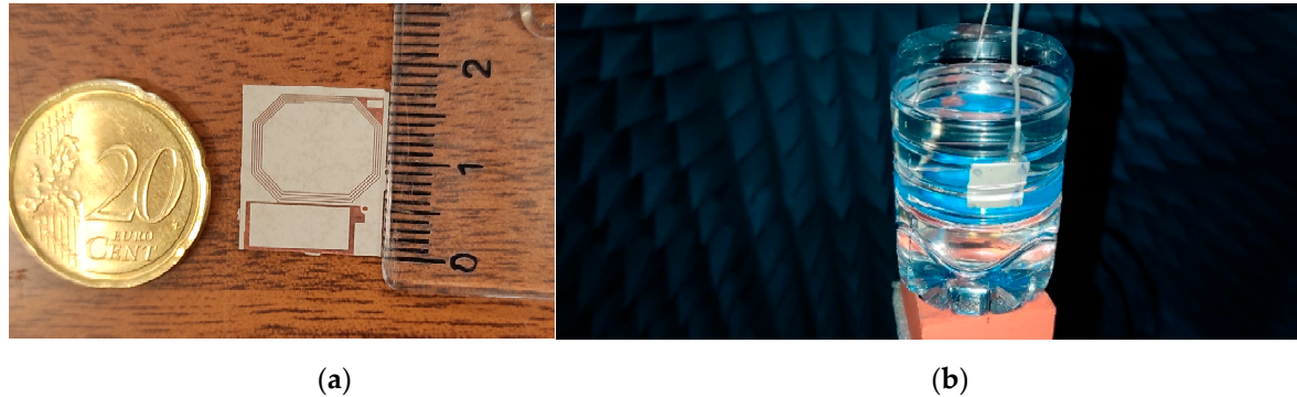
Figure 15. Fabricated dual-band antenna: (a) face view and size; (b) immersed in mixed skin-mimicking liquid inside the anechoic chamber.
