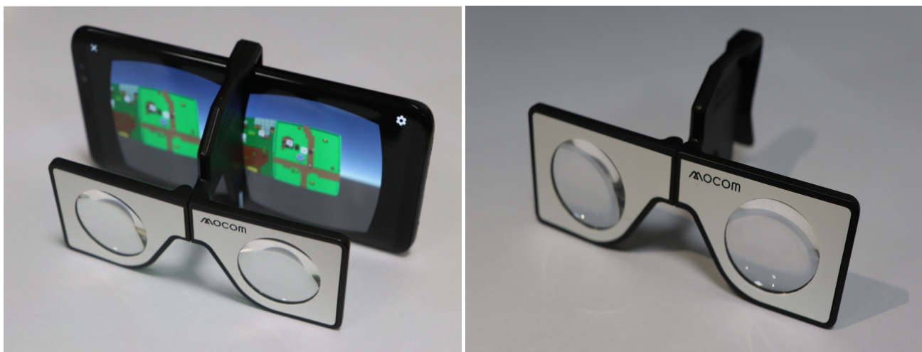
Figure 2. Smartphone based XR with clip-on lenses (left), the lenses itself (right).
