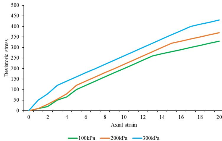
Figure 4. Clay deviatoric stress curves under different confining pressures.
