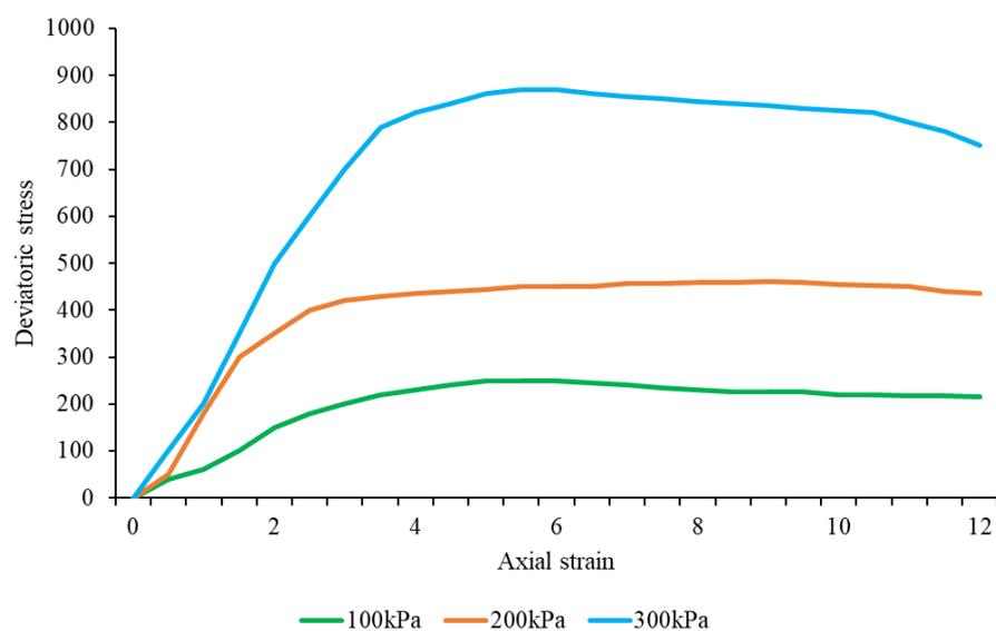
**Figure 3.** Deviatoric stress curves of sandy soil under different confining pressures.
