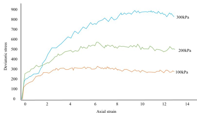
Figure 5. PFC simulation deviatoric stress curves of different sandy soils.
