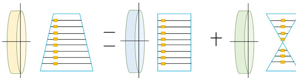
**Figure 2.** Equivalent force model of end-reinforced soil.
