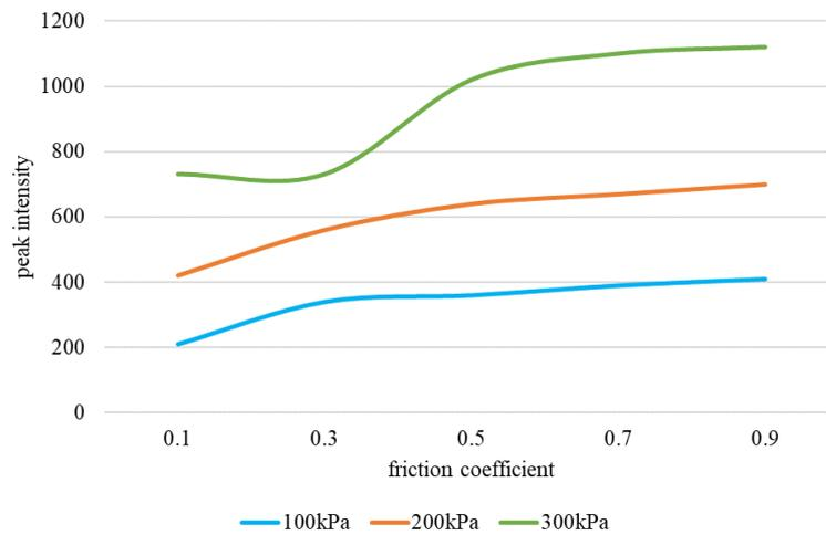
Figure 6. Relationship between particle friction coefficient and peak strength.
