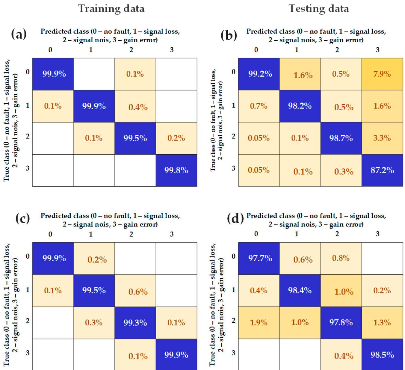
**Figure 17.** Confusion matrixes with percentage results for training and testing data for tested structure 30-10-2 for Output1(phase A) (a,b) and Output2(phase B) (c,d) in experimental studies.
