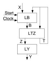
Figure 2. Structural diagram of MPY Mealy FSM.
