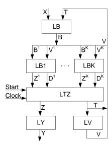
**Figure 3.** Structural diagram of  $MP_TY$  Mealy FSM.
