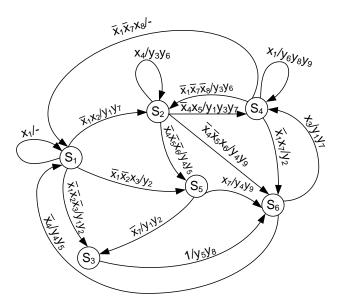
**Figure 4.** State transition graph of Mealy FSM *A*1.
