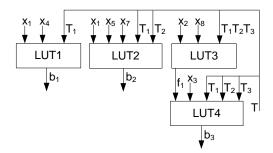
**Figure 8.** Circuit of block LB for Mealy FSM  $MP_TY(A1)$ .
