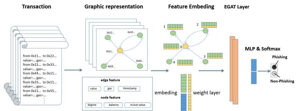
Figure 1. The framework of phishing account detection method based on EGAT.
