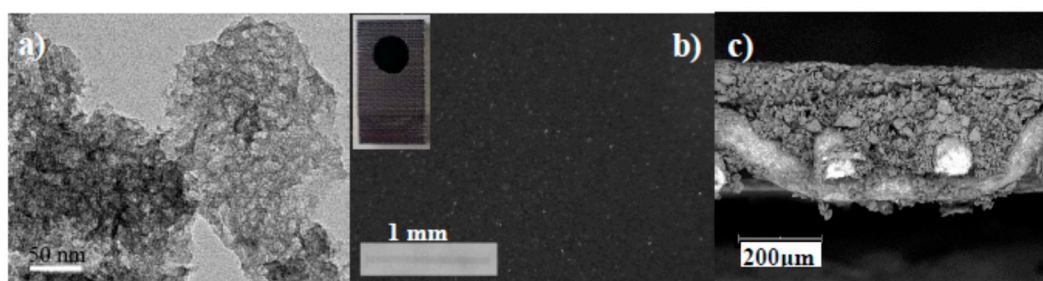
Figure 4. MC material and derivative MC/Ti CEs. (a) Representative transmission electron microscopy (TEM) image, (b) top view image of the front side of a MC-4/Ti CE with the photograph in the inset, (c) scanning electron microscope (SEM) image of cross-section of MC-4/Ti CE [31]. (Reproduced from Ref. [31], 10.1021/acs.jpcclett.6b01356, with permission.)
