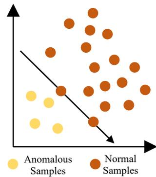
**Figure 2.** The illustration of OCSVM. It tries to find a hyperplane to separate the normal samples from the anomalous samples. The hyperplane, in particular, has the greatest distance to the origin.
