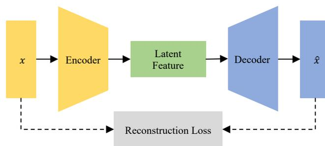
**Figure 1.** The architecture of an AE. The encoder compresses a original input  $x$  into a latent feature, and then the decoder reconstructs it from the latent feature.
