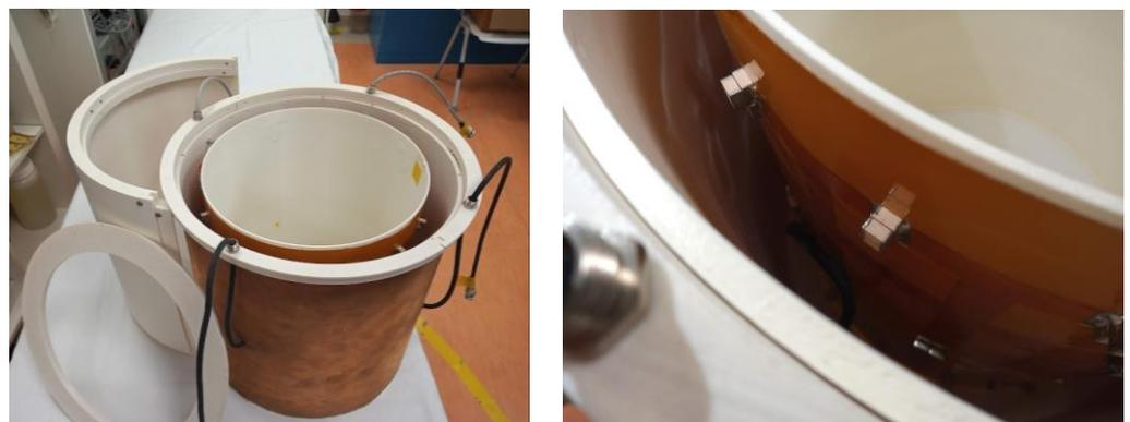
**Figure 10.** The four-ring DT-RF prototype view after removing the external case (left). Detail of the coil structure with two of the four rings visible (right).
