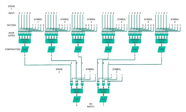
Figure 3. The 2-stage cascaded pattern identifier.
