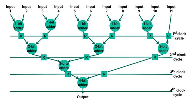
Figure 1. Adder tree for an 11-bit model.
