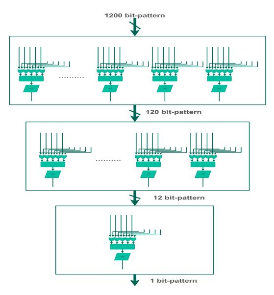
Figure 4. The 3-stage cascaded pattern identifier.
