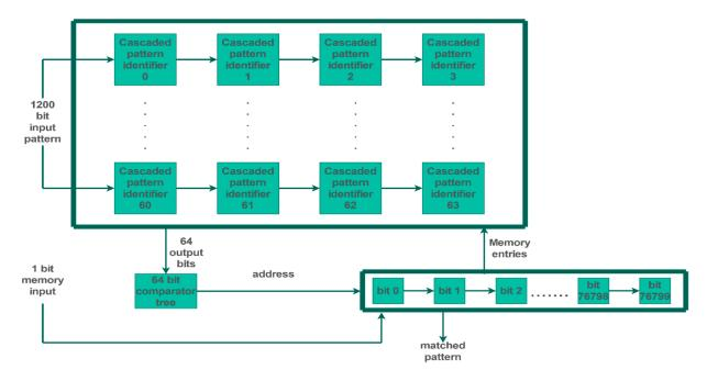
Figure 5. Pattern-matching circuit.
