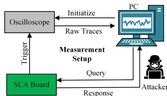
**Figure 2.** Overview of the SCA trace acquisition platform.
