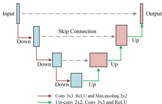
**Figure 3.** The U-Net architecture of our denoising model.
