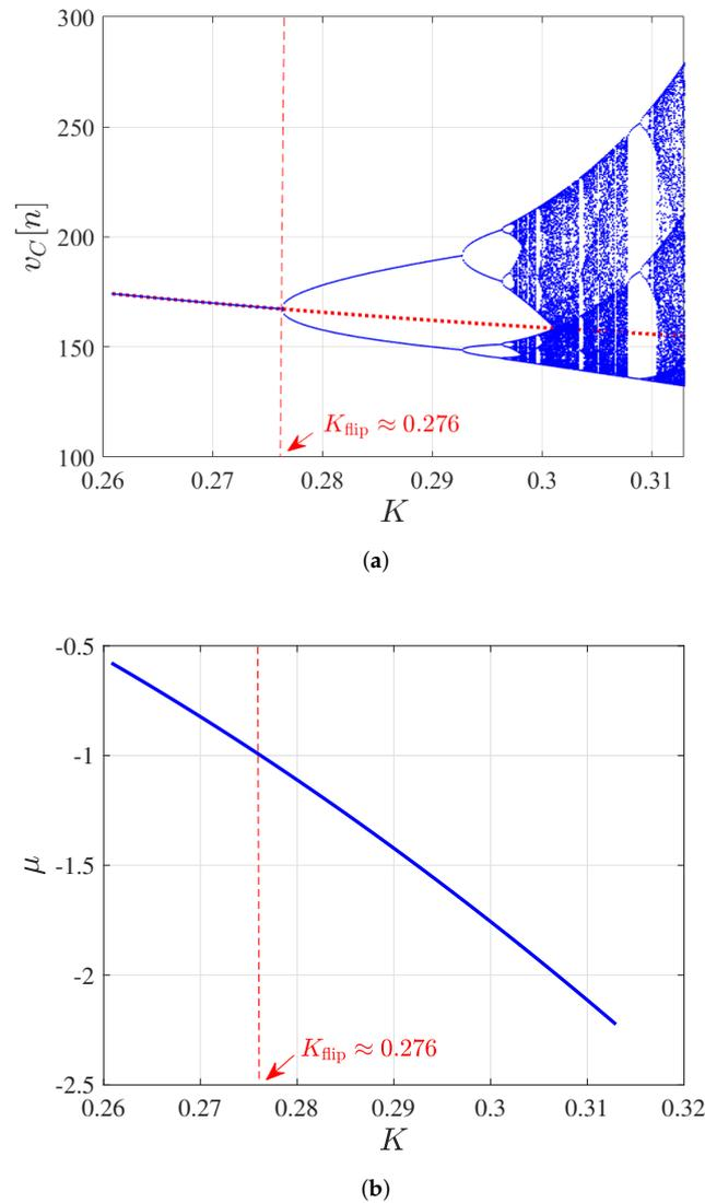
**Figure 13.** (a) Bifurcation diagram of the open–loop-DCM-operated boost converter with a CPL obtained using the approximated discrete–time model. The evolution of the fixed point is also represented by the dotted line. (b) Characteristic multiplier  $\mu$ .
