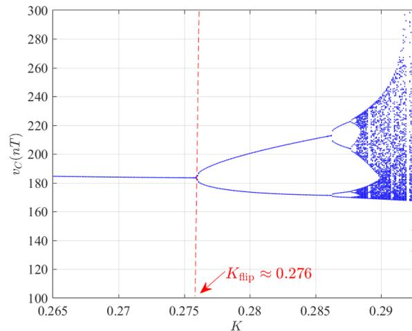
**Figure 10.** Bifurcation diagram of the DCM-operated boost converter with a CPL obtained using the PSIM<sup>®</sup> software.
