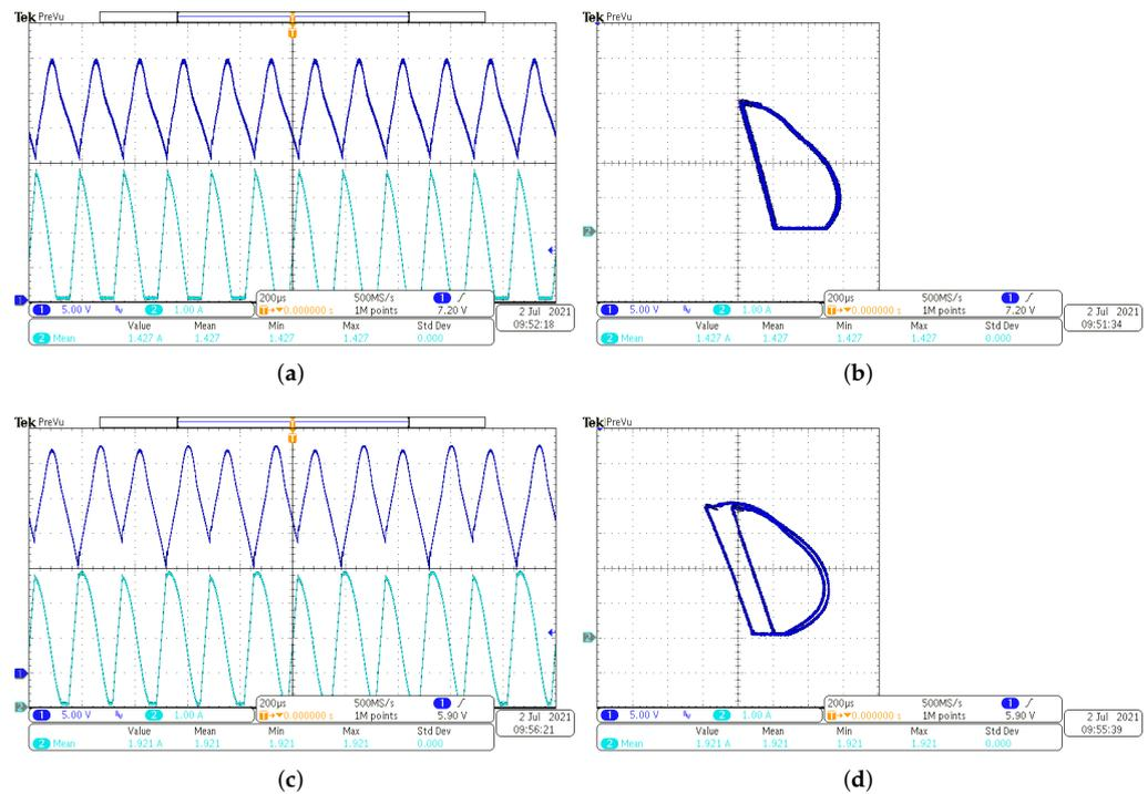
**Figure 4.** waveforms of an open-loop boost converter operating in DCM loaded by an ideal CPL. (a,b)  $P = 28\text{ W}$ : stable periodic regime, (c,d)  $P = 30\text{ W}$ : subharmonic oscillation due to period-doubling bifurcation.
