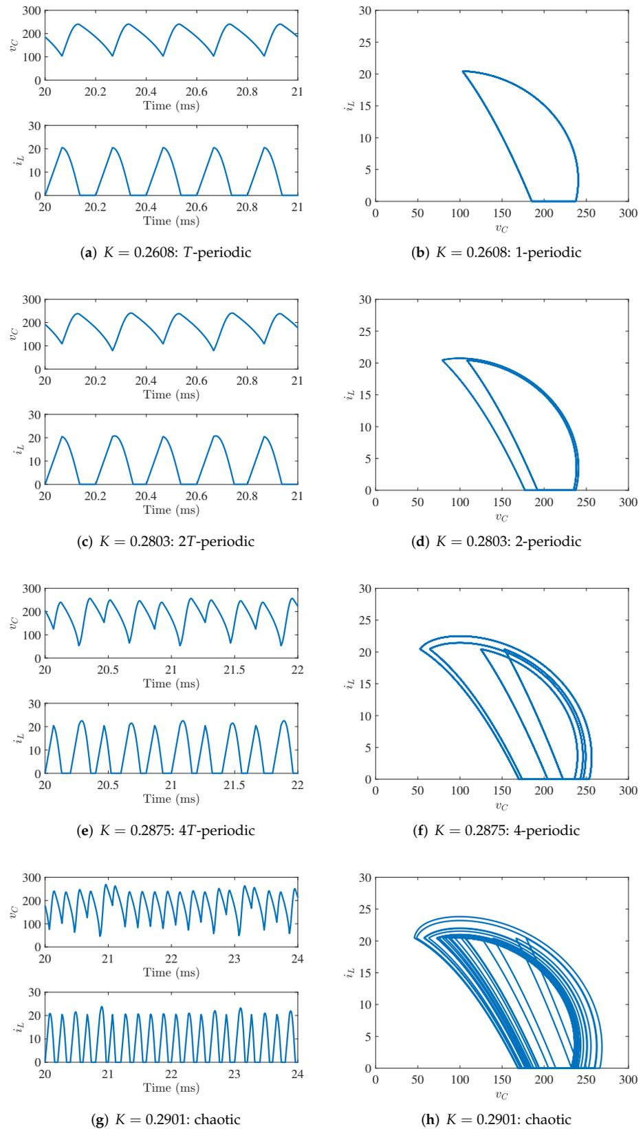
**Figure 11.** Time domain waveforms of the capacitor voltage and the inductor current for different dynamical behaviors obtained from the switched model of an open-loop-DCM-operated boost converter implemented in the PSIM<sup>®</sup> software.
