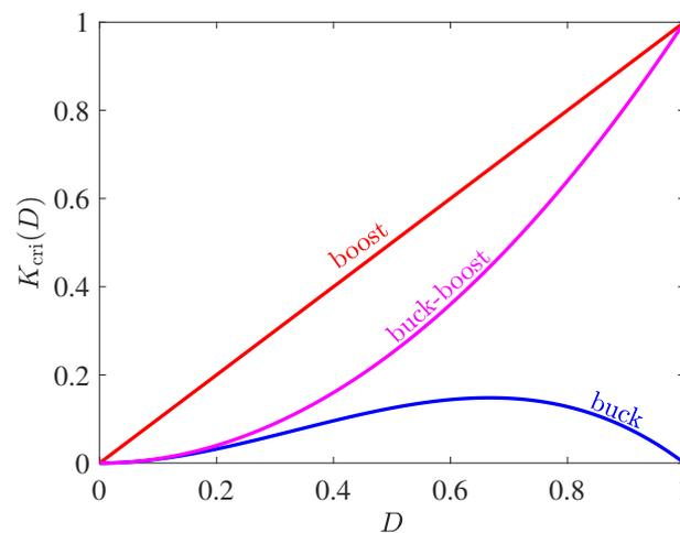
**Figure 7.** The critical value  $K_{\text{cri}}$  of  $K$  at the boundary CCM–DCM for elementary switching converters loaded by a CPL. For a specific value of  $D$ , if  $K > K_{\text{cri}}(D)$ , CCM takes place, and if  $K < K_{\text{cri}}(D)$ , DCM occurs.
