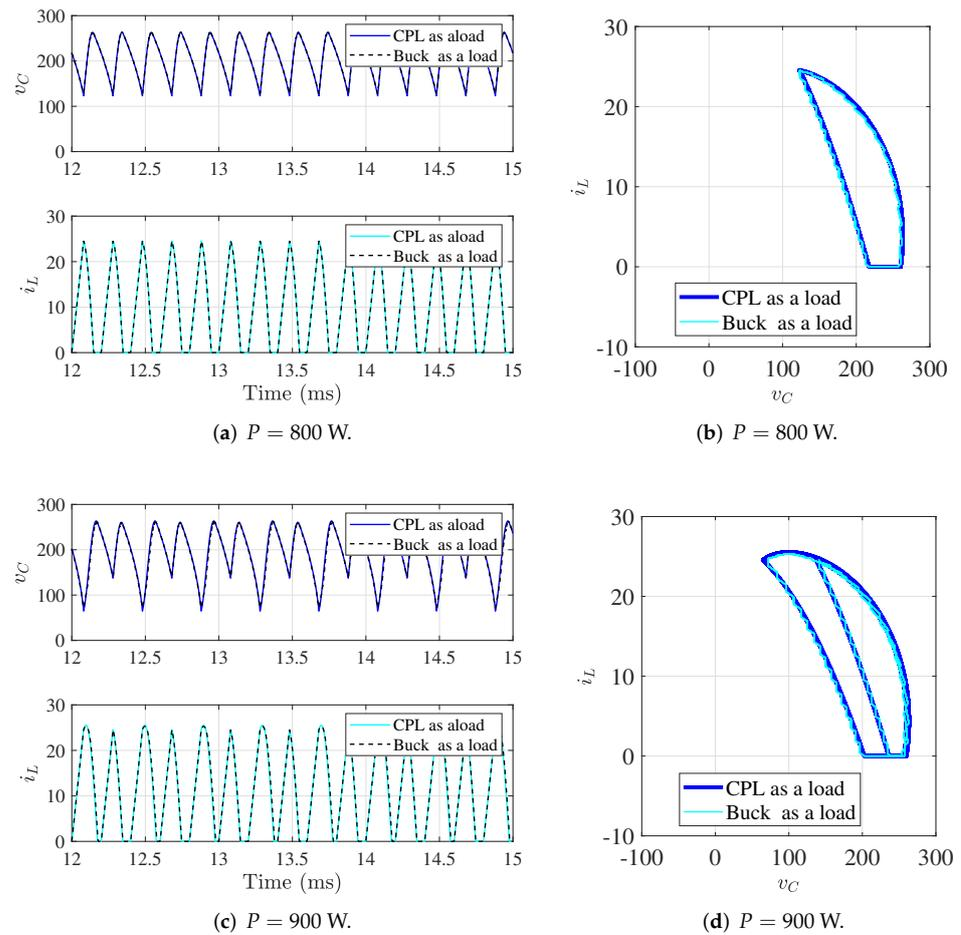
**Figure 2.** Behavior of an open-loop boost converter operating in DCM loaded by a tightly regulated buck converter and by an ideal CPL. (a, b)  $P = 800$  W: stable periodic regime, (c, d)  $P = 900$  W: subharmonic oscillation.
