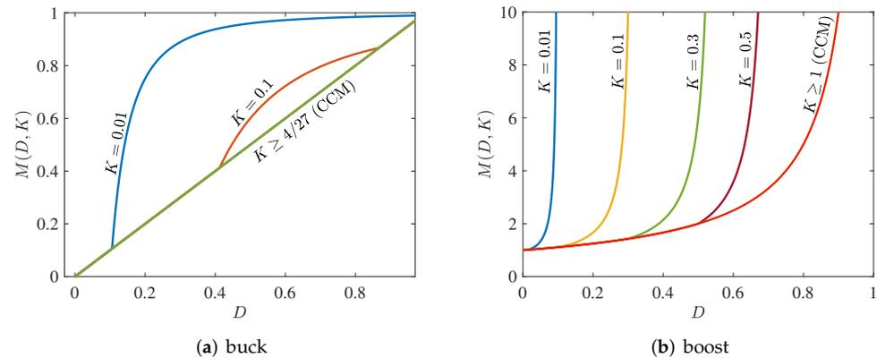
**Figure 9.** The conversion gain  $M(D, K)$  for the buck and the boost converter for different values of dimensionless parameter  $K$ . The conversion gain for CCM is also shown for comparison.
