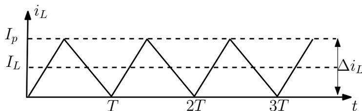
Figure 6. Steady-state inductor current  $i_L$  at the boundary of CCM–DCM for any elementary converter.
