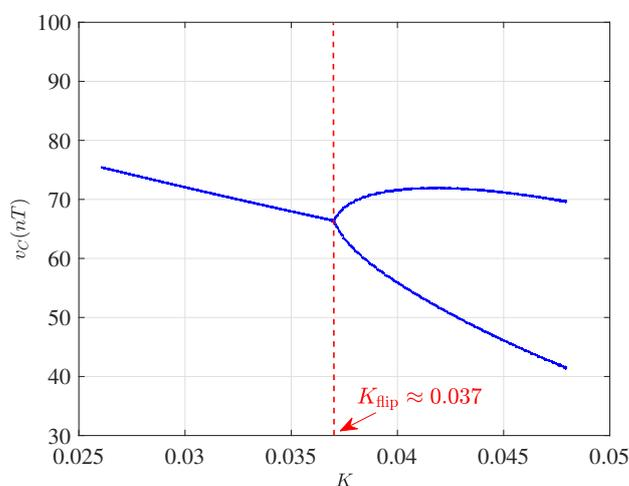
**Figure 12.** Bifurcation diagram of the DCM-operated buck converter with a CPL obtained using the PSIM<sup>®</sup> software.
