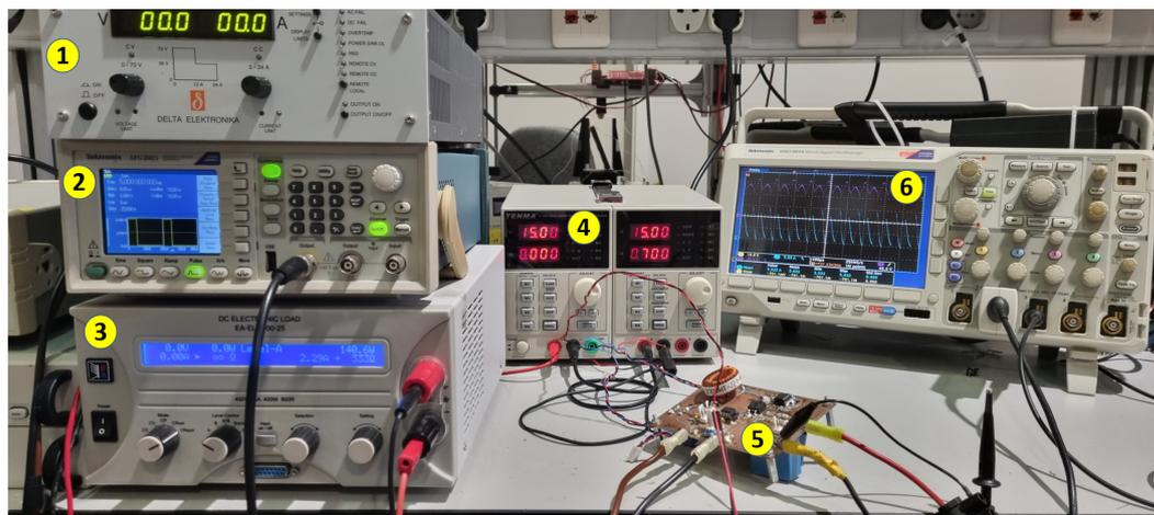
**Figure 3.** The experimental setup to observe period-doubling bifurcation in an open-loop boost converter with a CPL. ① Power supply, ② Function generator. ③ Electronic load. ④ Power supply. ⑤ Boost converter circuit. ⑥ Oscilloscope.
