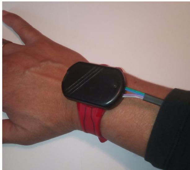
**Figure 4.** The sensing device on the participant's wrist.
