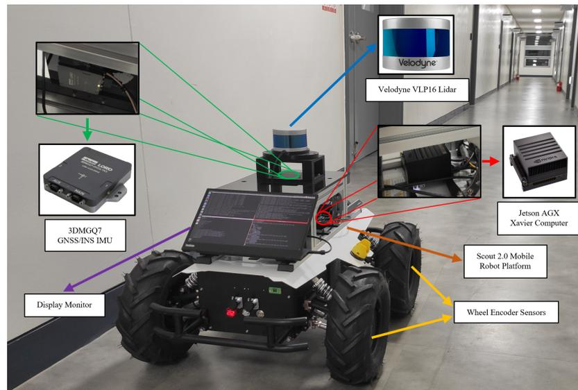
**Figure 4.** AGV configuration.
