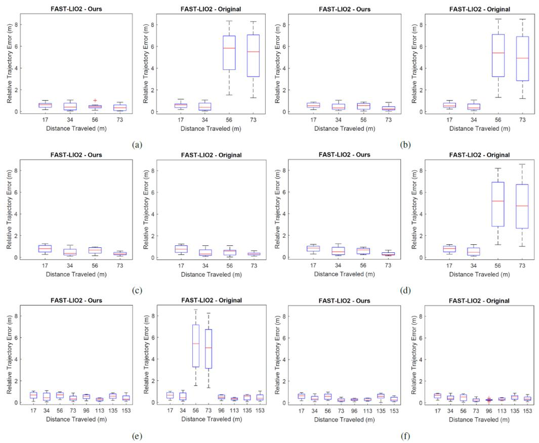
**Figure 7.** RTE results of the original and improved FAST-LIO2 in the flat terrain section of the tunnel environment: (a–d) single-loop runs, and (e,f) double-loop runs.
