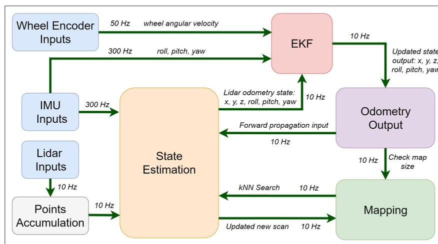
Figure 3. Overview of the modified FAST-LIO2 SLAM algorithm.
