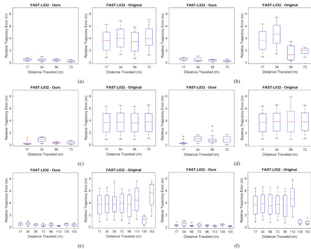
**Figure 9.** RTE results of the original and improved FAST-LIO2 in the inclined terrain section of the tunnel environment: (a–d) single-loop runs, and (e,f) double-loop runs.
