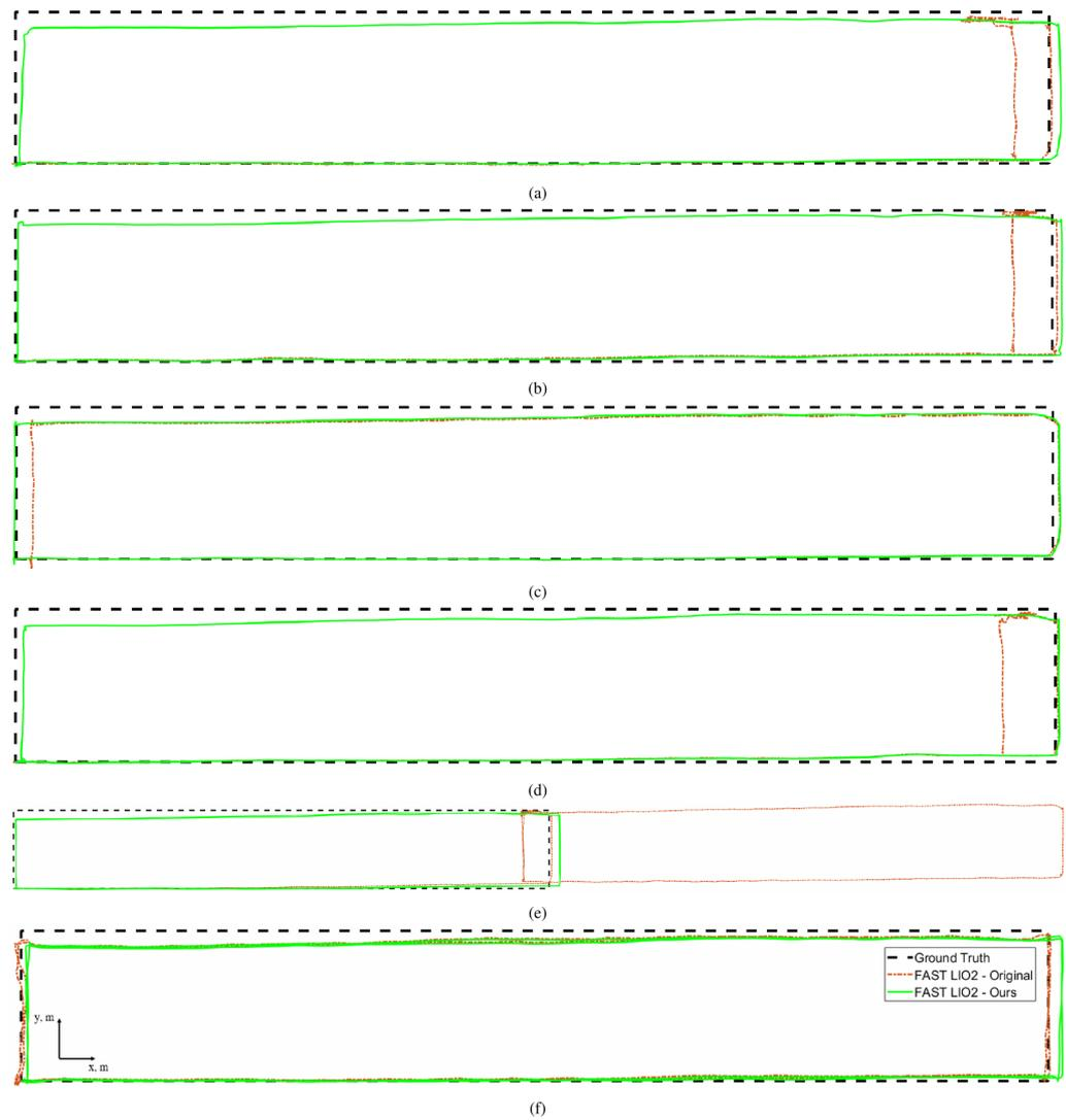
**Figure 6.** Estimated trajectory path comparison between the original and improved FAST-LIO2 in a flat terrain section of the tunnel environment: (a–d) single-loop runs, and (e,f) double-loop runs.
