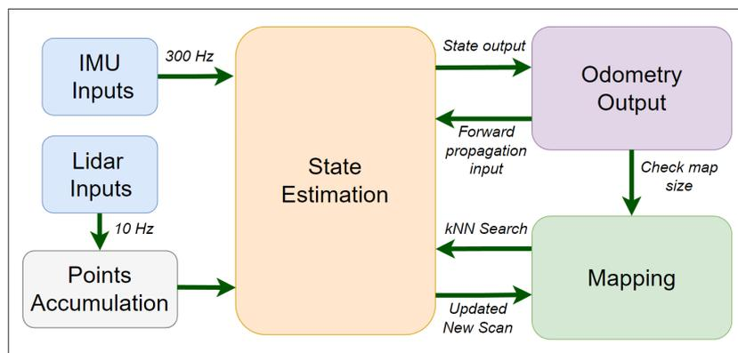
Figure 1. Simplified system overview of the original FAST-LIO2 SLAM algorithm.
