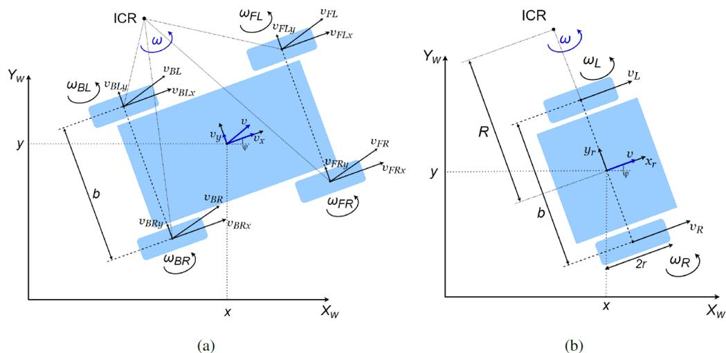
Figure 2. Motion model: (a) skid steering, and (b) two-wheel differential drive.
