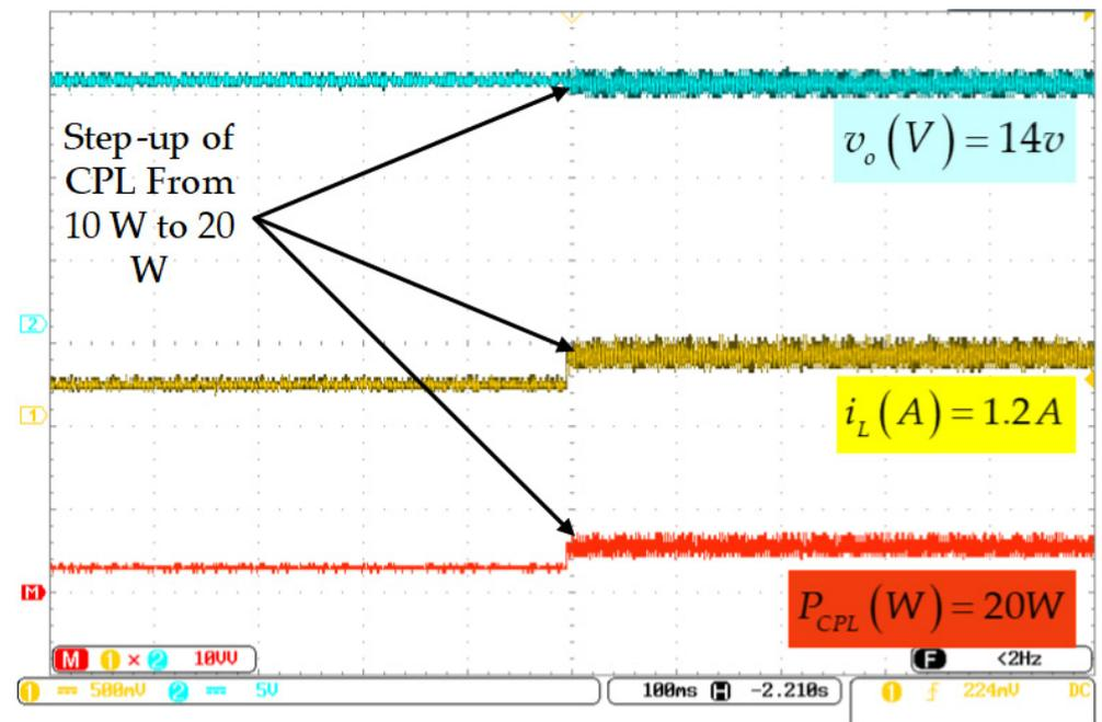
**Figure 16.** Experimental results for increased power demand of the CPL from 10 W to 20 W.
