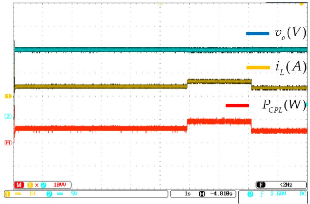
**Figure 15.** Experimental results: Time evolution of the output voltage and the output current against variable change in the CPL.
