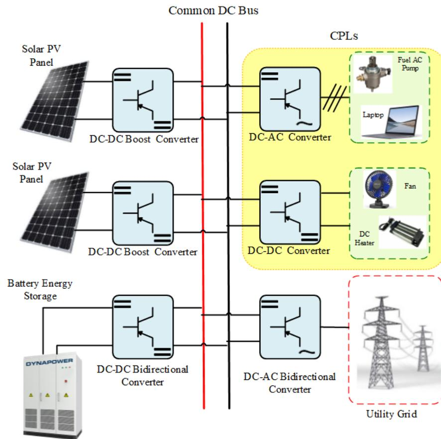
Figure 1. Structure of DC microgrid.
