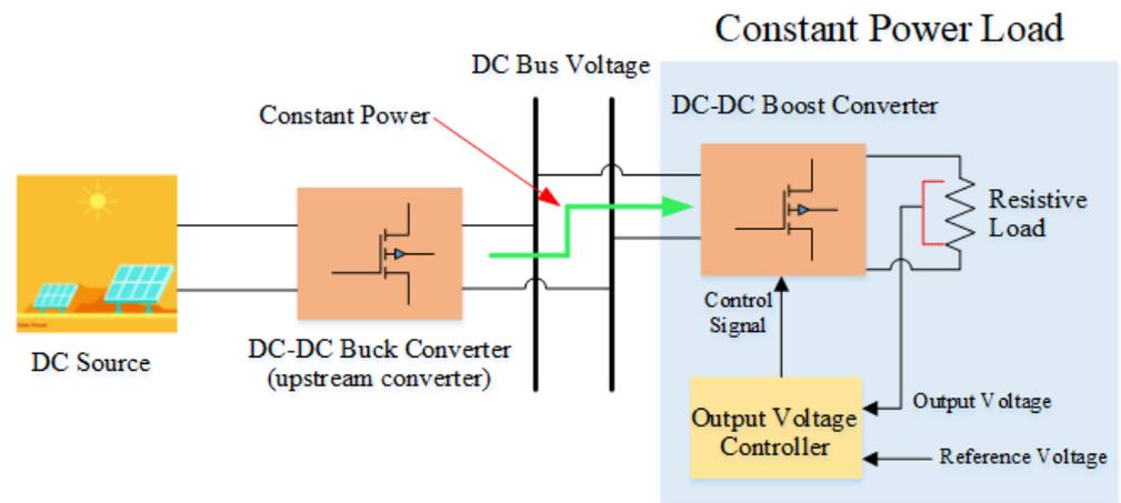
Figure 2. A cascaded structure of a buck converter feeding a voltage-controlled boost converter (operating as a CPL).
