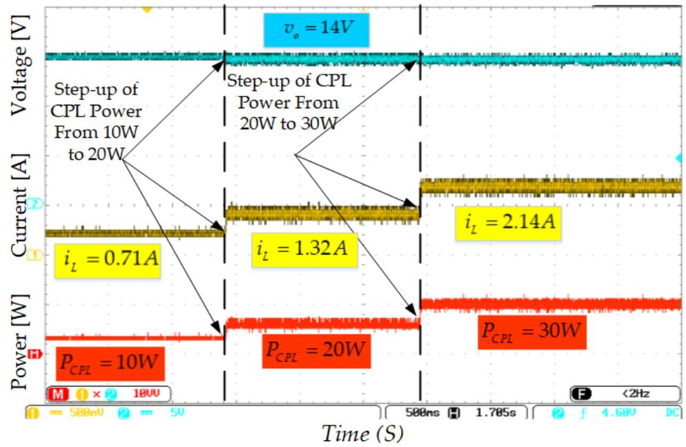
Figure 18. Experimental results of various step changes in the power absorbed by a CPL.
