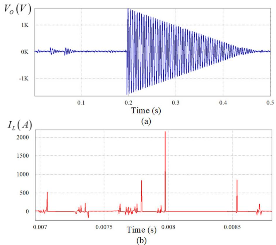
Figure 5. Behavior of the output current and voltage of a buck converter supplying a CPL ( $v_{in} = 28$  V,  $C = 220$   $\mu$ F,  $L = 20$  W,  $P_{CPL} = 20$  W, and  $d = 0.5$ ). (a) output voltage, (b) output current.
