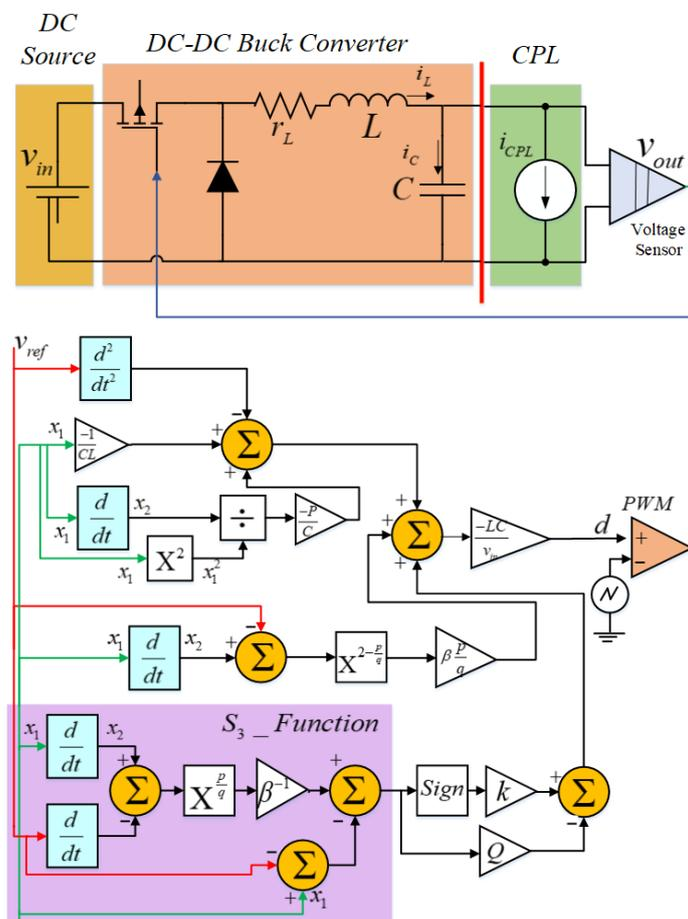
Figure 8. Block diagram of the NTSM controller applied for a buck converter supplying a CPL.
