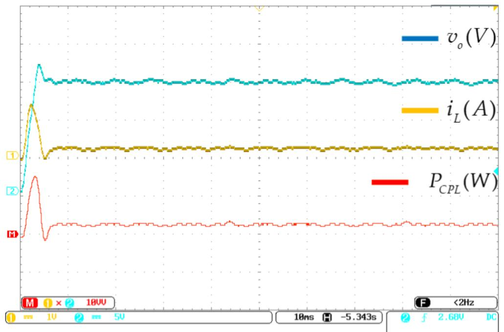
**Figure 14.** Experimental results: Time evolution of the output voltage, output current and power consumed by the CPL.
