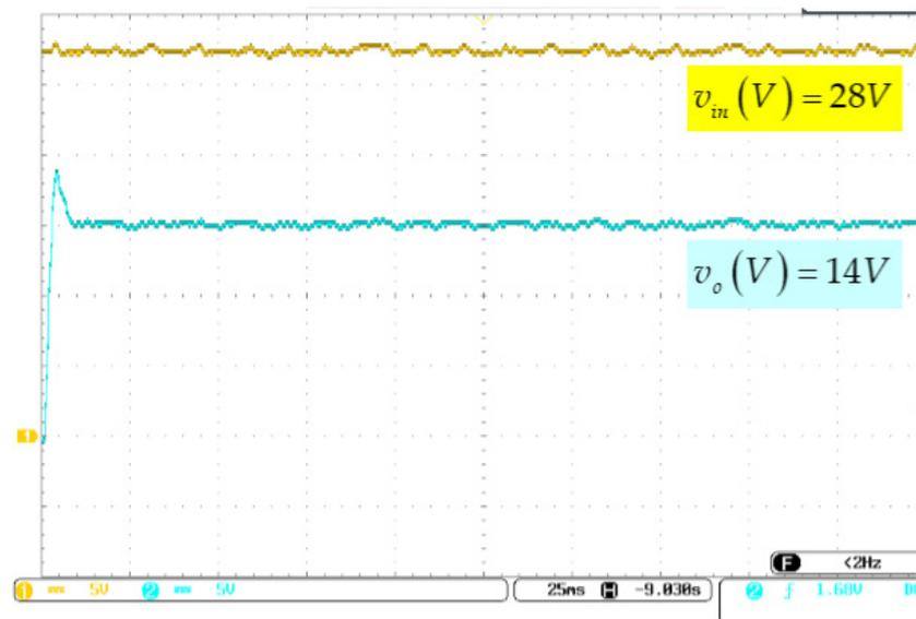
Figure 19. Experimental results of output voltage without changes in the input voltage.
