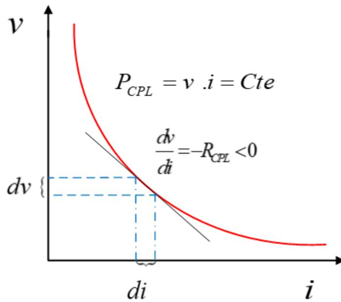
Figure 4. Incremental negative impedance behavior of a CPL.
