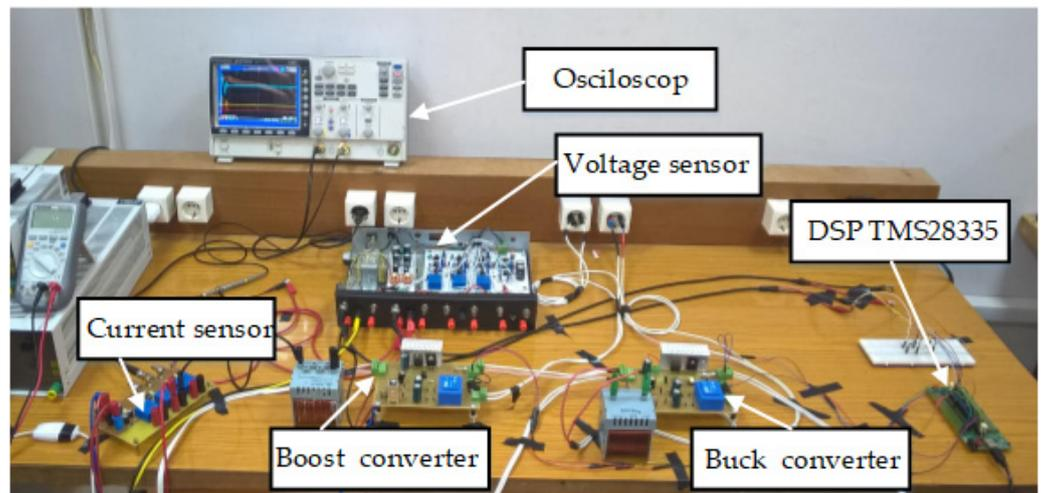
**Figure 13.** Experimental setup of the studied system.
