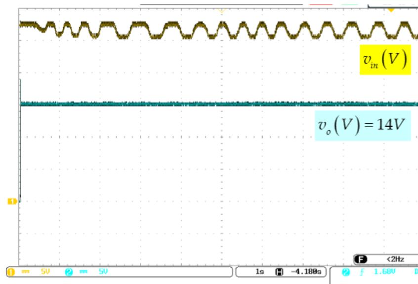
Figure 20. Experimental results of output voltage under the input voltage variation test.
