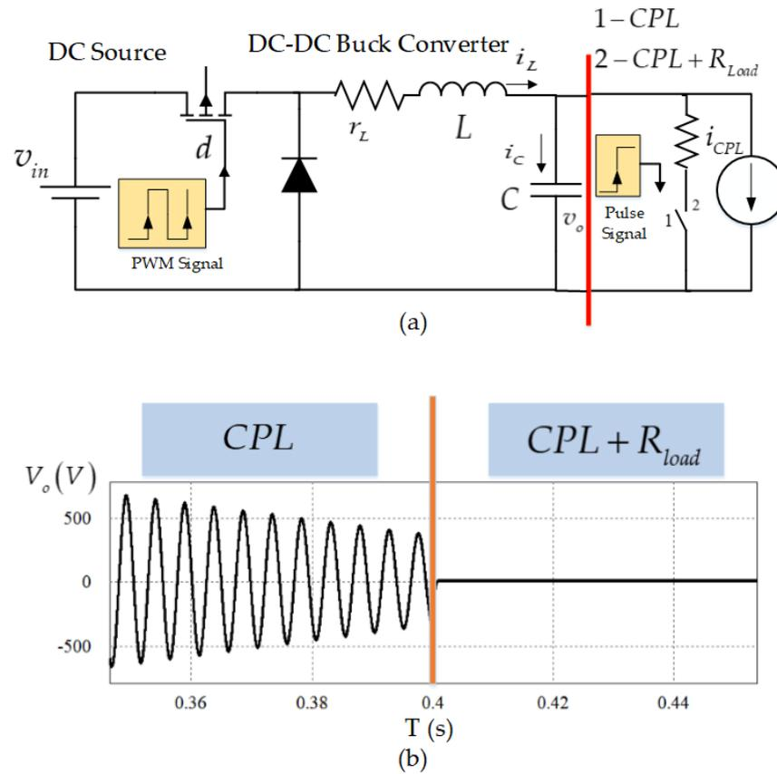
**Figure 6.** The influence of passive loads on the output voltage oscillations generated by the CPL. (a) A buck converter feeding two types of loads, (–1): CPL alone. (–2): CPL + R, (b) simulation result.
