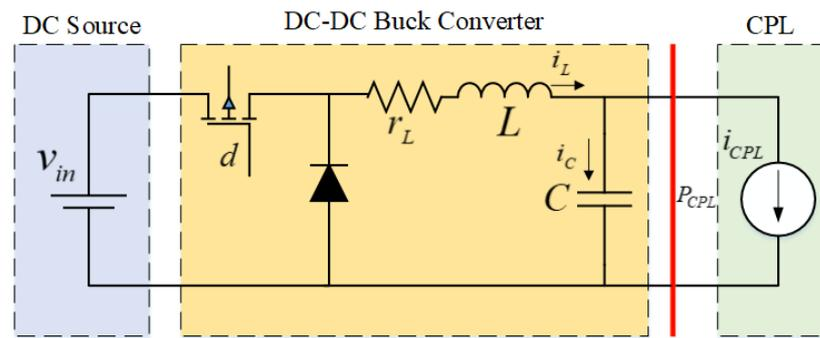
**Figure 3.** Equivalent circuit model of a buck converter supplying a CPL.
