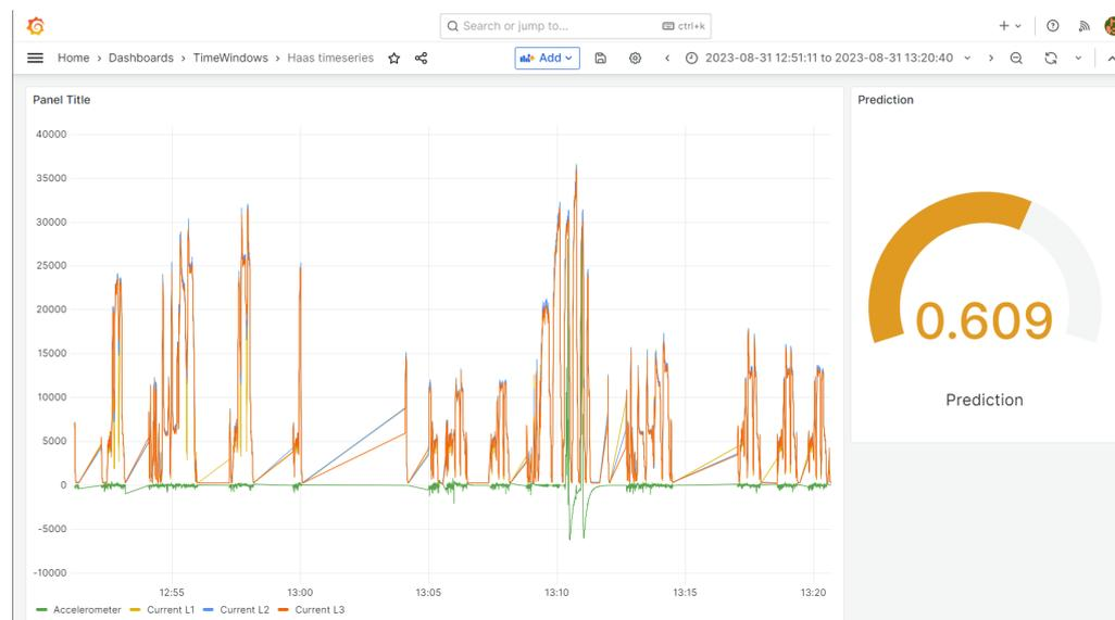
**Figure 13.** Visualization of a single experiments on a CNC machine along with the result of the predictions that determined the probability of problems with the machine.
