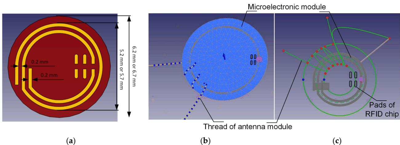
**Figure 5.** Model of coupling system in bead-shaped RFIDtex tag: (a) detailed diagram of two-loop chip's coupling circuit; (b) model with one turn in coupling circuit of microelectronic module; (c) designing process of model with two turns in coupling circuit of microelectronic module.
