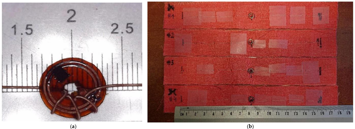
**Figure 9.** Experiment sample H1-H4: (a) example of coupling system; (b) four examples of RFIDtex transponder.
