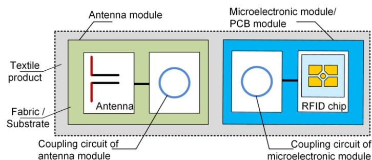
**Figure 2.** Idea for RFIDtex transponder.
