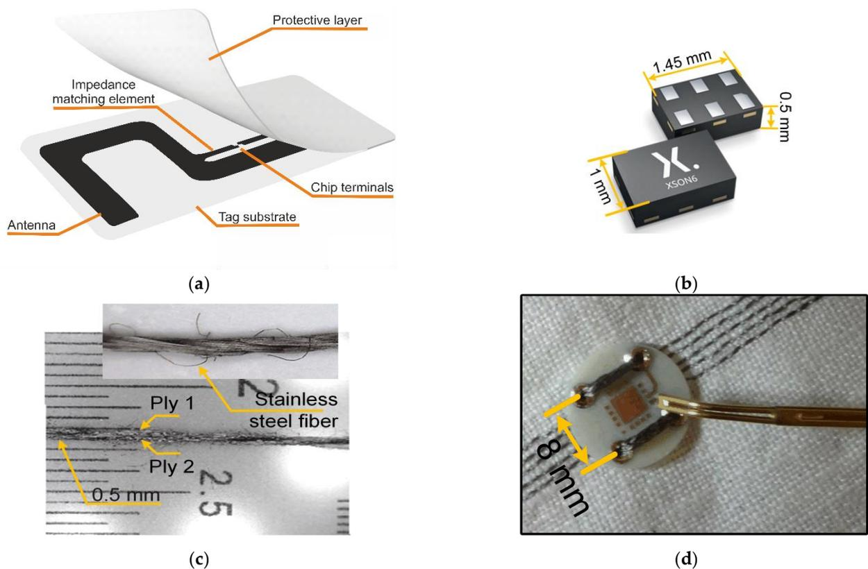
**Figure 1.** Designing RFIDtex transponder: (a) example of typical RFID tag design; (b) example of contemporary encapsulation of RFID chip; (c) conductive Adafruit 2 ply stainless thin thread; (d) example of galvanic connection between electronic module and conductive yarn system under laboratory tests.
