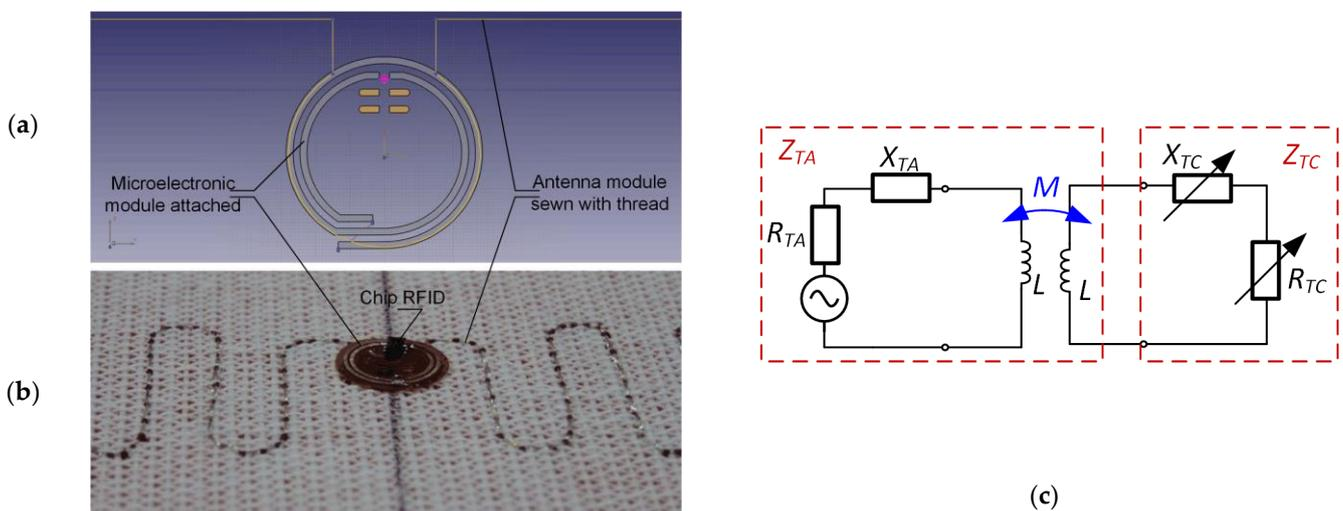
**Figure 4.** RFIDtex transponder according to Figure 3a: (a) classical model; (b) sample under tests; (c) diagram of electrical equivalent of RFIDtex transponder.
