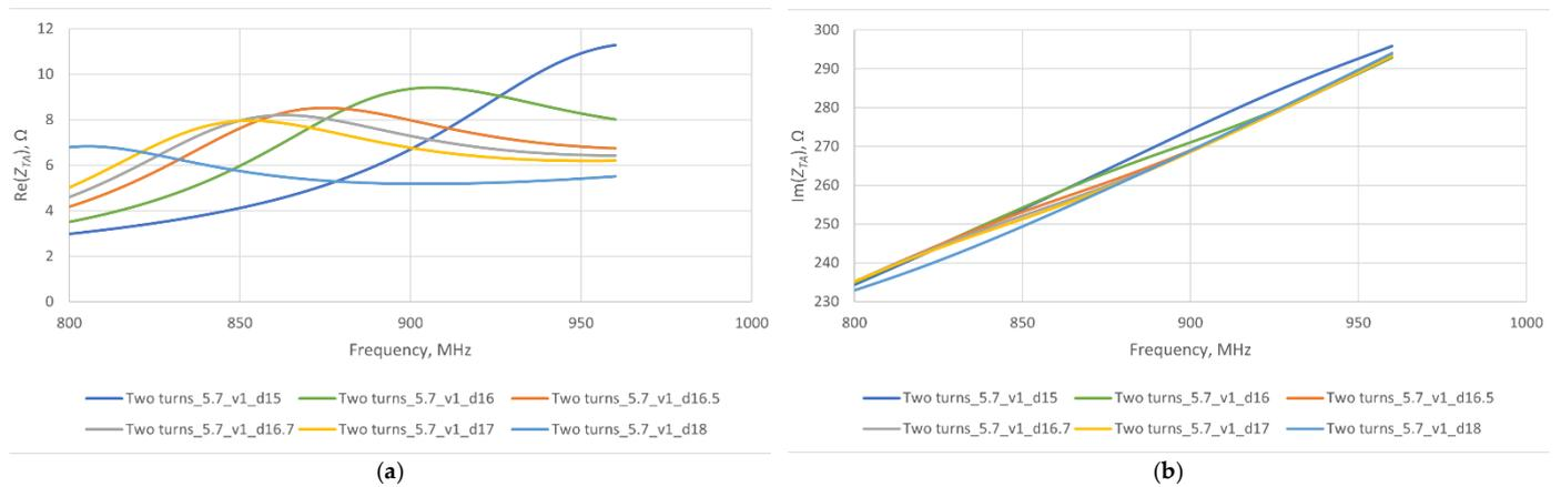
**Figure 8.** Antenna impedance  $Z_{TA}$  calculations for various length of antenna dipole: (a) real part of  $Z_{TA}$ ; (b) imaginary part of  $Z_{TA}$ .
