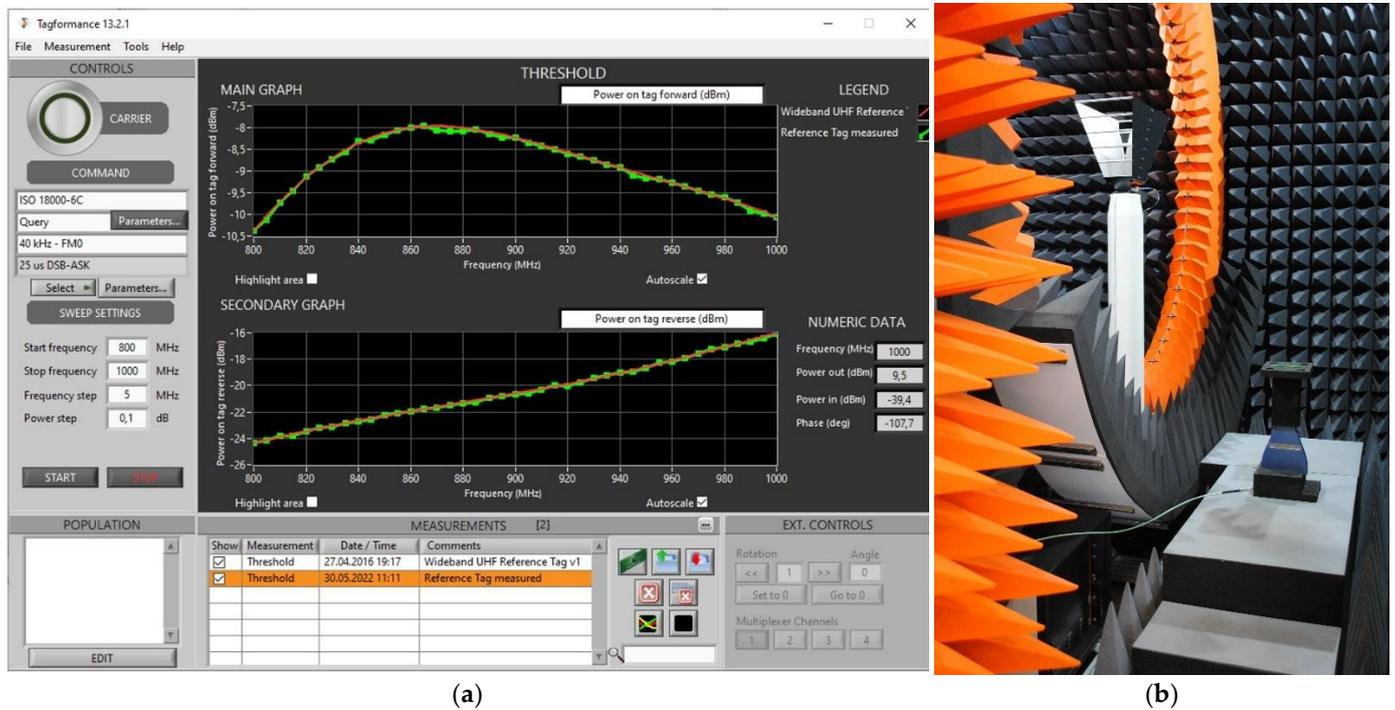
**Figure 10.** Experimental stand: (a) data condition in Voyantic Tagformance Pro development tool; (b) MVG anechoic chamber.
