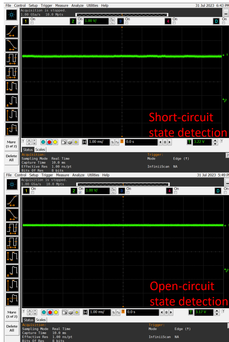
Figure 19. The optrode detection module experiment result. Two nodes of the detection module output digital voltage “1” in open-circuit and short-circuit states, respectively.
