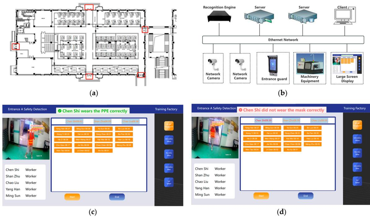
Figure 15. (a) Factory layout; (b) system deployment diagram; (c) system display interface for workers wearing PPE correctly; (d) system display interface for workers wearing PPE incorrectly.
