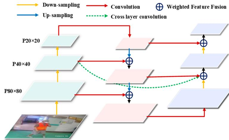
Figure 5. The architecture of BiFPN.
