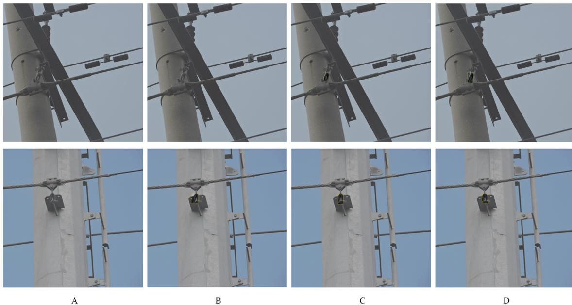
**Figure 8.** Visual detection results of small target fittings under various methods. The first and second rows depict the visual inspection results of a ball eye and a shackle, respectively. A is the U-Net, B is the U-Net combined with the DGCNN, C is the BRA-UNet, and D is the UD-Net.
