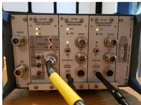
Figure 22. Illumination of the indicator LED on the front panel of the GX 526 amplifier unit.
