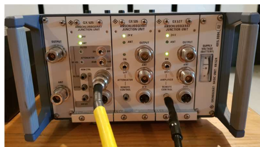
Figure 23. Illumination of the indicator LED on the GX 527 amplifier unit.
