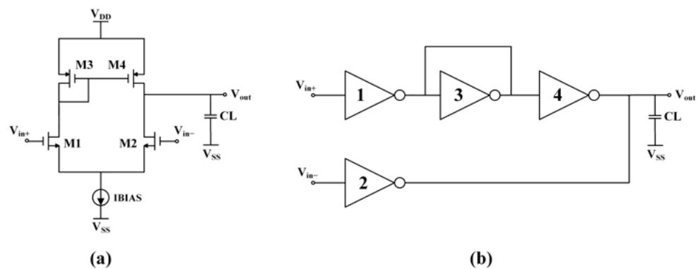
**Figure 6.** Conventional (a) and inverter-based (b) single-stage OTA.
