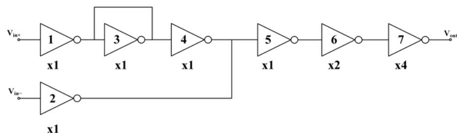
**Figure 7.** Schematic of the inverter-based OTA in [43].
