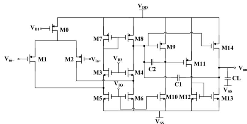
Figure 1. Schematic of the three-stage CMOS OTA operating in the subthreshold region proposed in [11].
