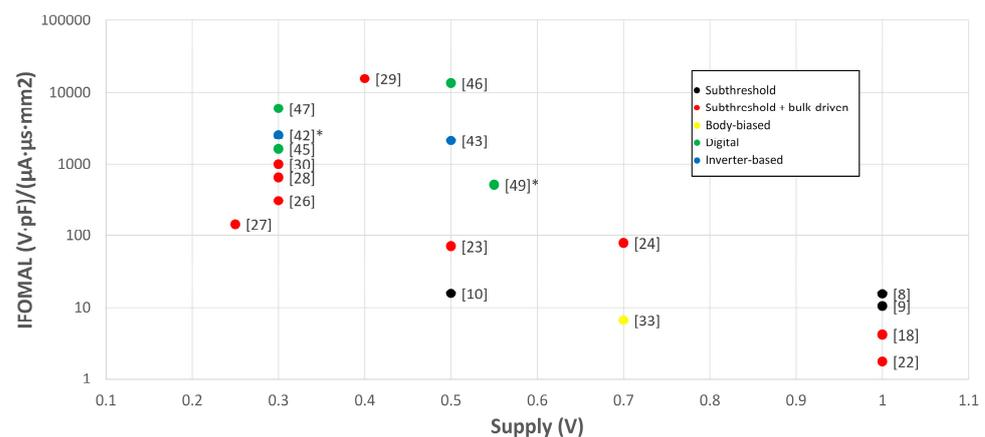
Figure 16.  $IFOM_{AL}$  vs. supply voltage (\* simulated).
