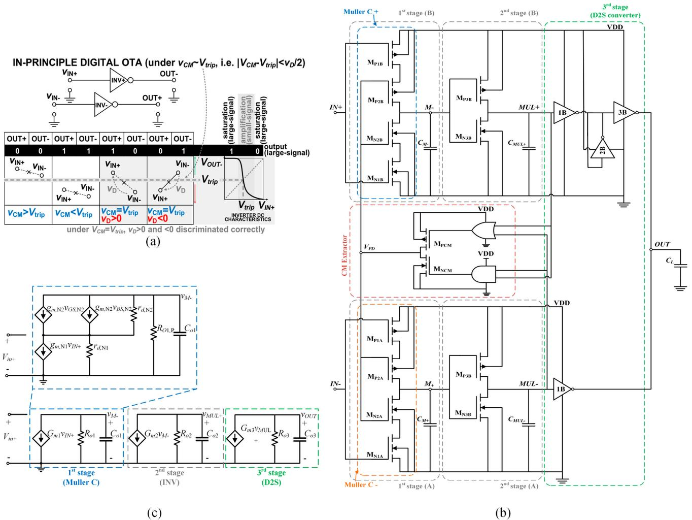
Figure 8. (a) Principle of operation of the DIGOTA introduced in [46]; (b) schematic and (c) small-signal model of the DIGOTA proposed in [51].
