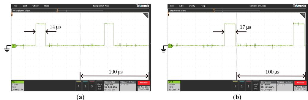
**Figure 11.** Experimental results of computational time consumption with different controls. (a) PI controller (b) Proposed method.
