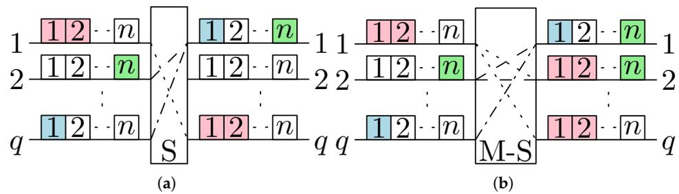
**Figure 3.** An example of (a) unicast and (b) multicast output-stage space switch operation; DSUs belonging to the same connection are marked with the same color.
