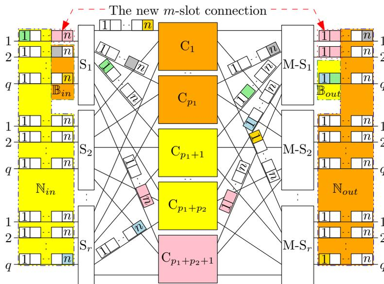
**Figure 7.** A scheme of sets of potential blocking and nonblocking connections in the M-SCS2 switching fabric (only important DSUs in interstage links are marked); DSUs belonging to the same connection are marked with the same color.
