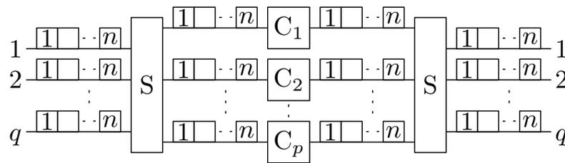
Figure 1. Symmetrical SCS1 switching fabric.
