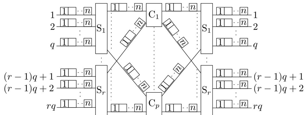
Figure 2. Symmetrical SCS2 switching fabric.
