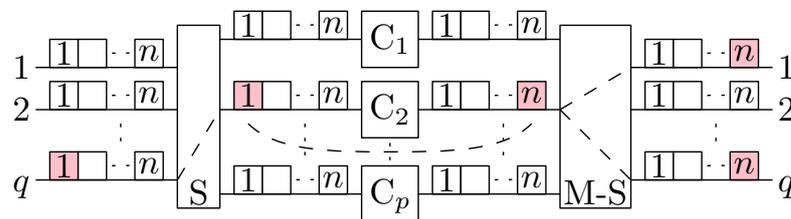
**Figure 4.** M-SCS1, a multicast switching fabric based on the SCS1 architecture with multicast capability in the third-stage switch and an example of a two-cast one-slot connection; DSUs belonging to the same connection are marked with the same color.
