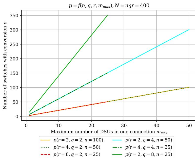
**Figure 14.** Number of switches with conversion in the middle stage versus  $m_{max}$  in M-SCS2 switching fabrics with  $N = nqr = 400$  and different values of  $r, q,$  and  $n$ .
