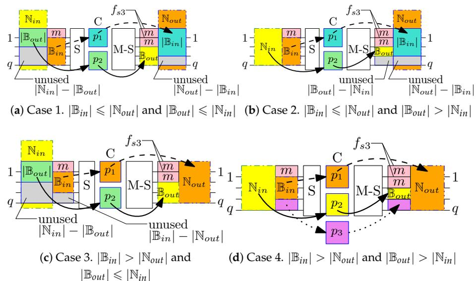
**Figure 8.** Four cases to determine the maximum number of blocked middle-stage switches; all cases are described later in the paper.
