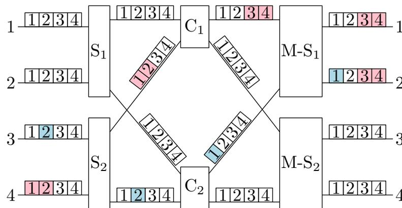
**Figure 5.** An illustration of the M-SCS2 switching fabric architecture, denoted  $M-SCS(q = 2, p = 2, r = 2, n = 4, f = 2)$ , along with an example showcasing two mutually blocking connections; DSUs belonging to the same connection are marked with the same color.
