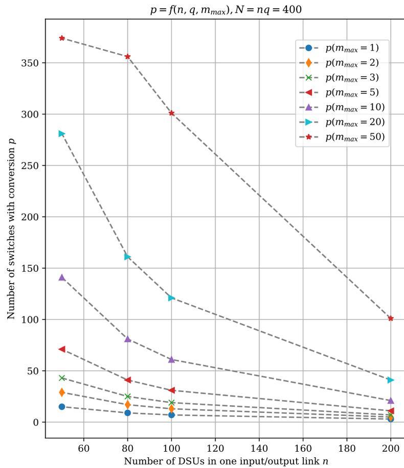
**Figure 13.** Number of switches with conversion in the middle stage of M-SCS1 switching fabrics with  $N = nq = 400$  and different values of  $m_{max}$  and  $q = 400/n$ .
