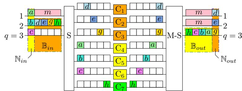
**Figure 11.** An example for Case 4 is a switching fabric with  $q = 3, n = 5, m = 4$ , and  $f_{s3} = 2$ ; DSUs belonging to the same connection are marked with the same color.
