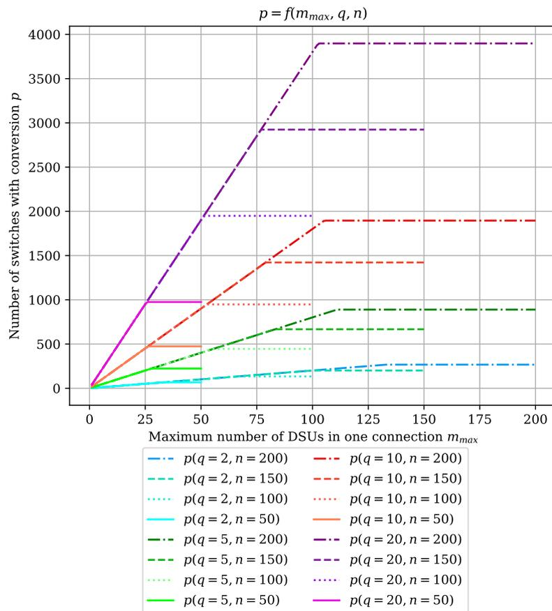
**Figure 12.** Number of switches with conversion in the middle stage of M-SCS1 switching fabrics with different values of  $q$  and  $n$ .
