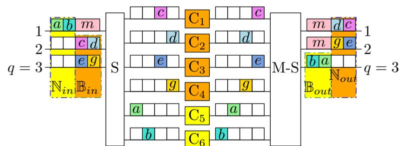
**Figure 9.** An example for Case 1 is a switching fabric with  $q = 3, n = 4, m = 2$ , and  $f_{s3} = 2$ ; DSUs belonging to the same connection are marked with the same color.
