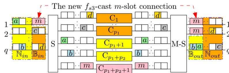
**Figure 6.** An example of sets of potential blocking and nonblocking connections in the M-SCS1 switching fabric for the new multicast connection; DSUs belonging to the same connection are marked with the same color.
