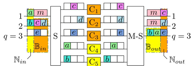
**Figure 10.** An example for Case 3 is a switching fabric with  $q = 3, n = 3, m = 2,$  and  $f_{s3} = 2$ ; DSUs belonging to the same connection are marked with the same color.
