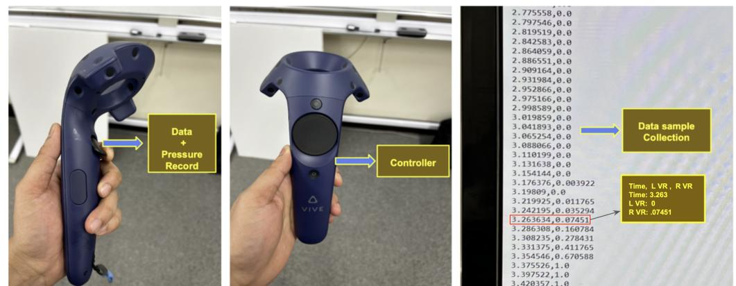
Figure 22. VR device remote for data collection.
