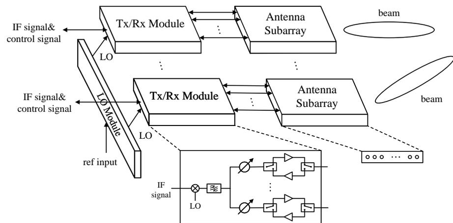
**Figure 2.** The architecture of the phased antenna array. Phase shifters, amplifiers and switches in Tx/Rx modules are controlled by the control signal, and the control circuit is omitted.
