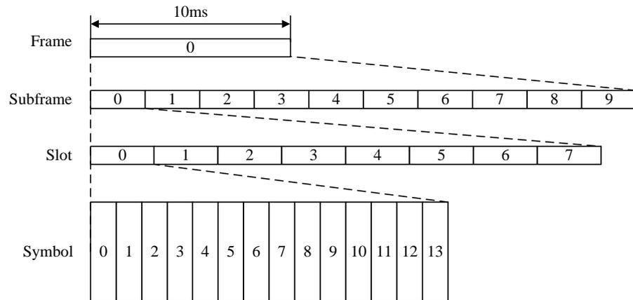
**Figure 8.** The frame structure. Each frame is divided into 80 slots. Each slot is further divided into 14 OFDM symbols.
