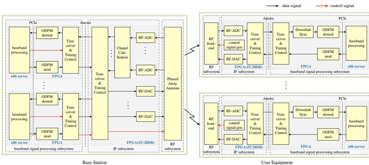
Figure 1. Overview of our proposed XL-MIMO testbed in the multi-UE scenario.
