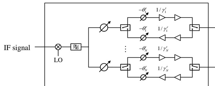
Figure 3. Modified Tx/Rx Module for transmitting and receiving calibration.
