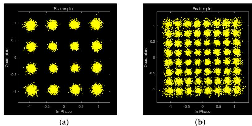
**Figure 12.** Received constellations under different modulation schemes. (a) Received constellation under 16-QAM modulation; (b) Received constellation under 64-QAM modulation.
