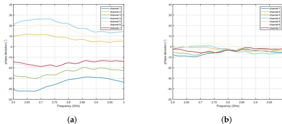
Figure 5. Phase deviations of each channel. The phase differences are reduced from about  $-40^\circ \sim 30^\circ$  to about  $-10^\circ \sim 4^\circ$ . (a) Phase deviations before calibration; (b) Phase deviations after calibration.
