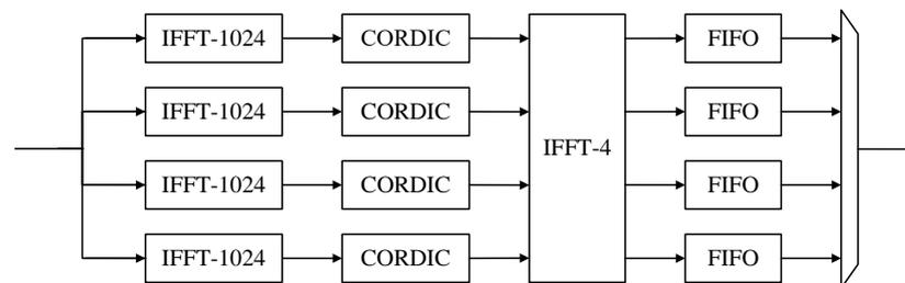
Figure 9. The architecture of parallel IFFT module.
