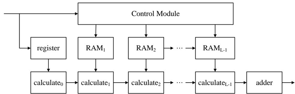
Figure 4. The architecture of channel calibration modules.
