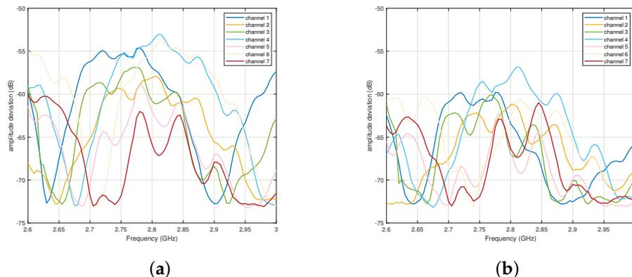
**Figure 6.** Amplitude deviations of each channel. The maximum amplitude deviations are reduced from about  $-53$  dB to less than  $-55$  dB. (a) Amplitude deviations before calibration; (b) Amplitude deviations after calibration.
