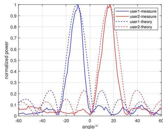
**Figure 11.** The measured and theoretical beam patterns of the given two users scenario.
