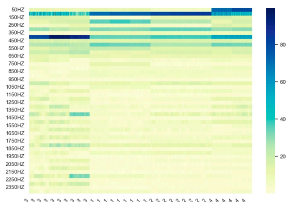
Figure 6. Clustering heat map of transformer vibration characteristics.
