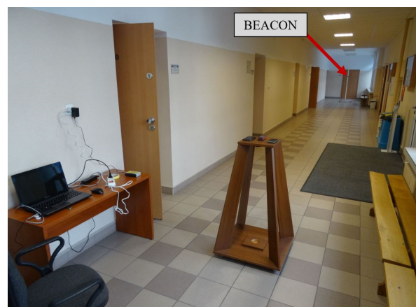
Figure 3. Setup for measuring the signal strength of indoor-located beacon.
