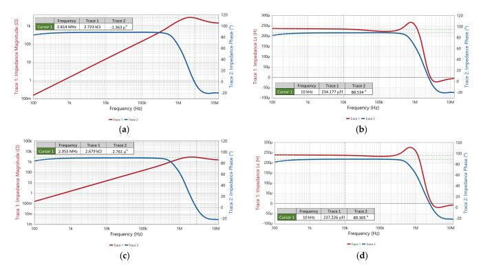
**Figure 6.** (a) Sample 2 impedance plot: red—impedance magnitude; blue—impedance phase; (b) sample 2 inductance plot: red—inductance value; blue—impedance phase; (c) sample 3 impedance plot: red—impedance magnitude; blue—impedance phase; red—impedance phase; (d) sample 3 inductance plot: red—inductance value, blue—impedance phase.
