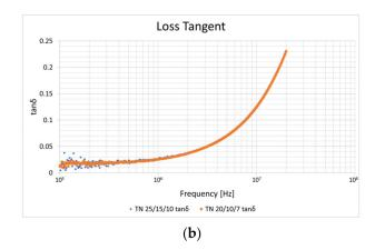
**Figure 13.** Coating-to-core permittivity and loss tangent characteristics. (a) Real and imaginary parts of complex permittivity: grey—real part of sample 2; yellow—imaginary part of sample 2; blue—real part of sample 3; orange—imaginary part of sample 3; (b) loss tangent: orange—sample 2; blue—sample 3.
