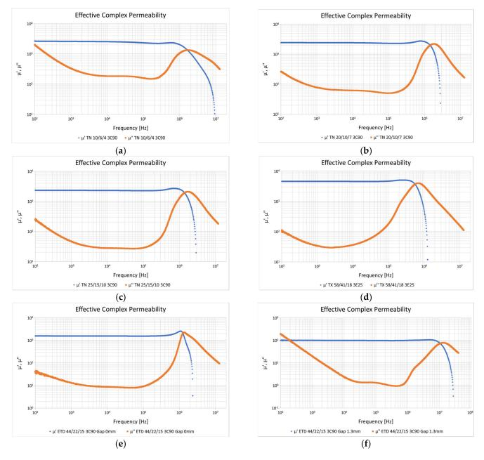
**Figure 4.** Effective complex permeability plots: blue—real part of complex permeability; orange—imaginary part of complex permeability; (a) sample 1; (b) sample 2; (c) sample 3; (d) sample 4; (e) sample 5; (f) sample 6.
