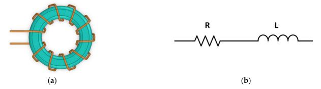
Figure 1. (a) Toroidal ferrite coil and (b) its equivalent simplified series model.
