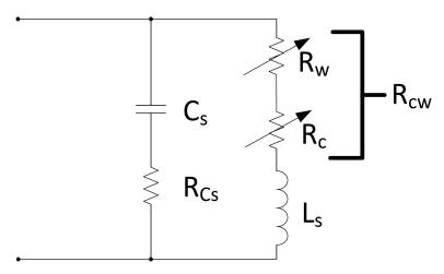
Figure 2. Series un-gapped high-frequency equivalent inductor model.
