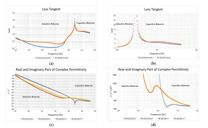
**Figure 14.** Sample 2 and sample 3 loss tangent and complex permittivity characteristics. (a) Loss tangent: orange—sample 2; blue—sample 3; (b) loss tangent—zoom at self-resonant frequency:
