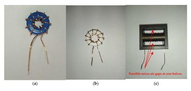
**Figure 5.** (a) Sample 2 used in verification of complex permeability characteristics; (b) sample 3 used in verification of complex permeability characteristics; (c) sample 5 with possible micro air gaps affecting complex permeability values.
