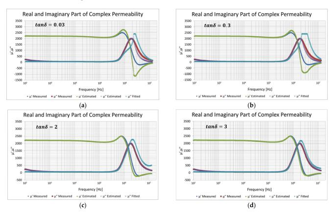
**Figure 9.** Sample 2 fitting convergence depending on loss tangent value: dark blue—real part of measured characteristic; green—real part of estimated characteristic; dark red—imaginary part of measured characteristic; purple—imaginary part of estimated characteristic; light blue—imaginary part of fitted characteristic; (a) loss tangent 0.03; (b) loss tangent 0.3; (c) loss tangent 2; (d) loss tangent 3.
