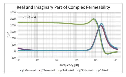
**Figure 8.** Sample 2 real and imaginary parts of complex permeability: dark blue—real part of measured characteristic; green—real part of estimated characteristic; dark red—imaginary part of
