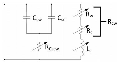
Figure 18. Improved series equivalent inductor model.
