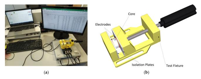
Figure 12. (a) Complex permittivity test-bench; (b) complex permittivity test fixture.
