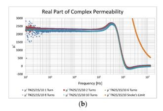
**Figure 15.** Sample 2 and sample 3 real part of complex permeability characteristics at different number of turns and Snoke's limit; (a) sample 2: blue—1 turn; red—2 turns; green—6 turns; violet—8 turns; light blue—10 turns; orange—Snoke's limit; (b) sample 3: blue—1 turn; red—2 turns; green—6 turns; violet—8 turns; light blue—10 turns; orange—Snoke's limit.
