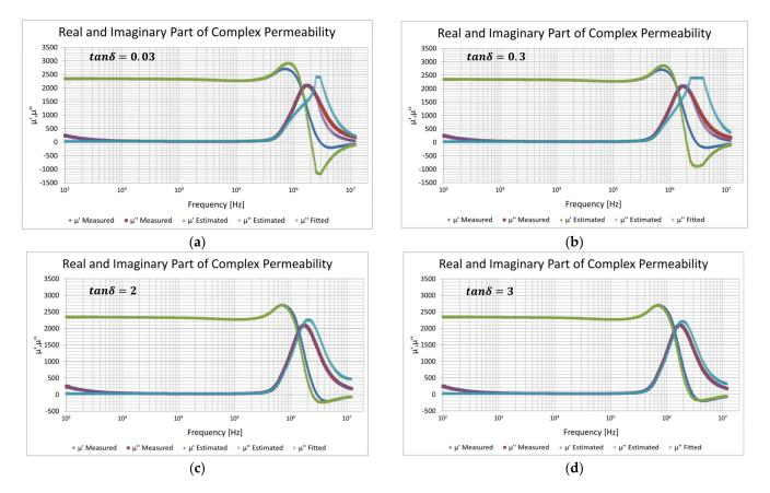
**Figure 11.** Sample 3 fitting convergence depending on loss tangent value: dark blue—real part of measured characteristic; green—real part of estimated characteristic; dark red—imaginary part of measured characteristic; purple—imaginary part of estimated characteristic; light blue—imaginary part of fitted characteristic; (a) loss tangent 0.03; (b) loss tangent 0.3; (c) loss tangent 2; (d) loss tangent 3.
