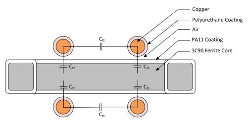
Figure 7. Sample 2 and 3 cross-section with highlighted turn-to-turn and turn-to-core capacitance.
