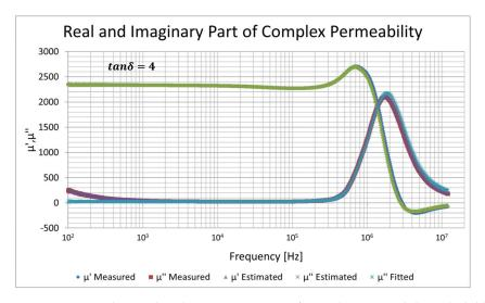
**Figure 10.** Sample 3 real and imaginary parts of complex permeability: dark blue—real part of measured characteristic; green—real part of estimated characteristic; dark red—imaginary part of measured characteristic; purple—imaginary part of estimated characteristic; light blue—imaginary part of fitted characteristic.
