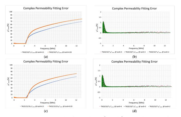
**Figure 19.** Relative fitting error between  $\mu''_{r_{measured}}$  and  $\mu''_{r_{estimated}}$  (a) sample 1: orange— $tand\delta = 0.03$ ; blue  $tan\delta = 0.3$ ; (b) sample 1: green— $tand\delta = 2$ ; grey— $tand\delta = 3$ ; red— $tand\delta = 4$ ; (c) sample 2: orange— $tand\delta = 0.03$ ; blue  $tan\delta = 0.3$ ; (d) sample 2: green— $tand\delta = 2$ ; grey— $tand\delta = 3$ ; red— $tand\delta = 4$ .
