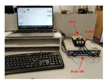
**Figure 3.** Complex permeability test-bench setup.
