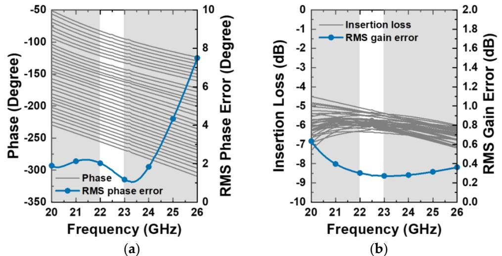
**Figure 7.** Simulated results: (a) phase and RMS phase error and (b) insertion loss and RMS gain error.
