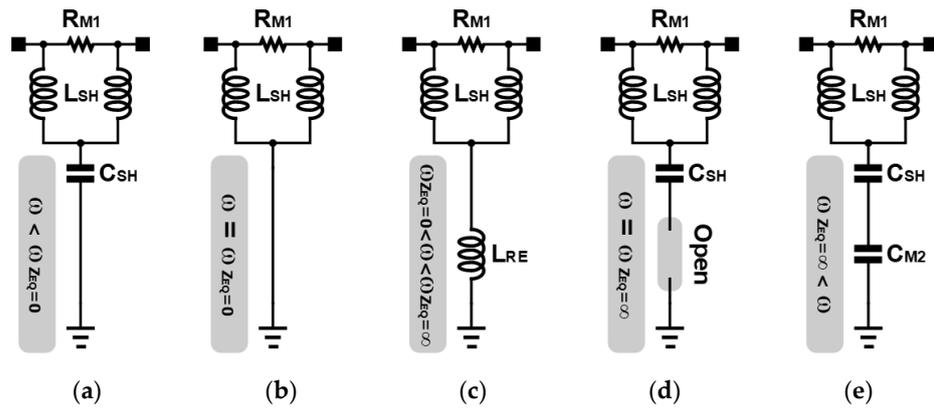
**Figure 2.** Equivalent circuits for pass mode according to frequency: (a)  $\omega < \omega_{Z_{EQ}=0}$ , (b)  $\omega = \omega_{Z_{EQ}=0}$ , (c)  $\omega_{Z_{EQ}=0} < \omega < \omega_{Z_{EQ}=\infty}$ , (d)  $\omega = \omega_{Z_{EQ}=\infty}$ , and (e)  $\omega_{Z_{EQ}=\infty} < \omega$ .
