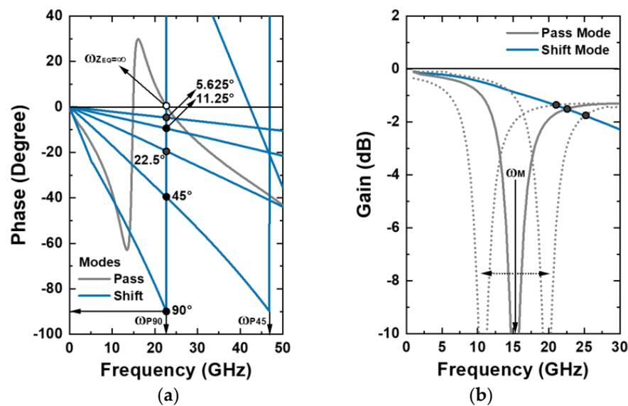
Figure 3. Conceptual diagrams for securing required (a) phase and (b) gain.
