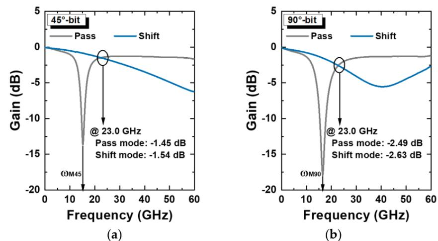
Figure 5. Simulated gains for shift and pass modes for (a) 45° and (b) 90° bits.
