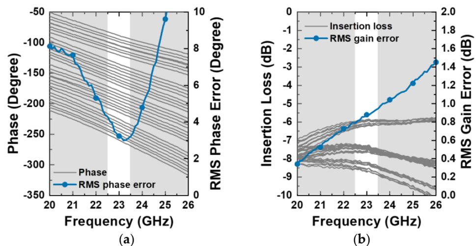
**Figure 9.** Measurement results: (a) phase and RMS phase error and (b) insertion loss and RMS gain error.
