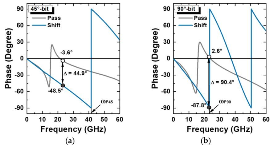
Figure 4. Simulated phases for shift and pass modes for (a) 45° and (b) 90° bits.
