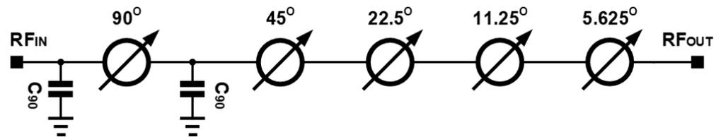
**Figure 6.** Overall structure of the designed phase shifter.
