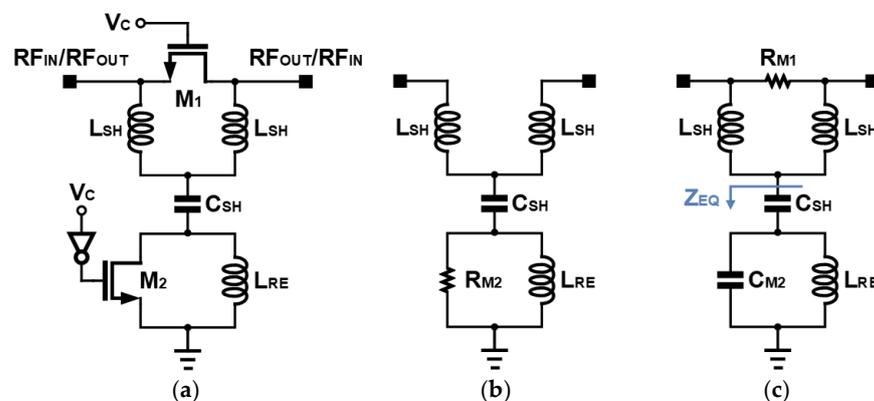
**Figure 1.** T-type structure: (a) schematic of the used T-type structure, and equivalent circuits for the (b) shift and (c) pass modes.
