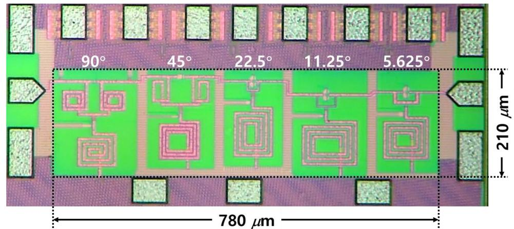
**Figure 8.** Chip photograph of the designed K-band CMOS phase shifter.
