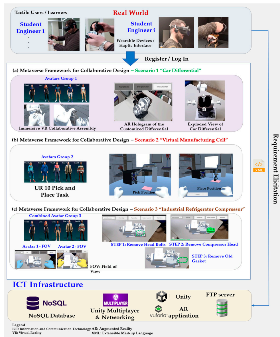
Figure 7. Collaborative design mixed reality case studies in the proposed platform immersive learning framework: (a) car differential; (b) virtual manufacturing cell; (c) industrial refrigerator compressor.
