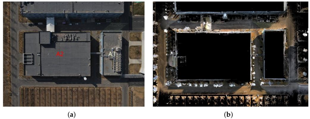
**Figure 2.** An example of mapping around the A2 building and A3 building of *Raytron Technology Co.* (called *Raytron*). (a) the color image depicting the mapping region taken from a top view by a DJI Mavic3 drone; (b) the mapping result (top view) of the proposed algorithm.
